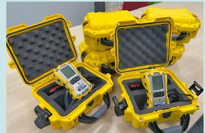
New MultiRAE lite gas detectors with upgraded sensors to meet the new WorkSafe New Zealand standards.
