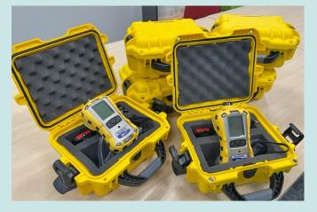
New MultiRAE lite gas detectors with upgraded sensors to meet the new WorkSafe New Zealand standards.
