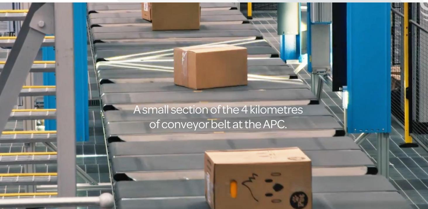
A small section of the 4 kilometres of conveyor belt at the APC.
