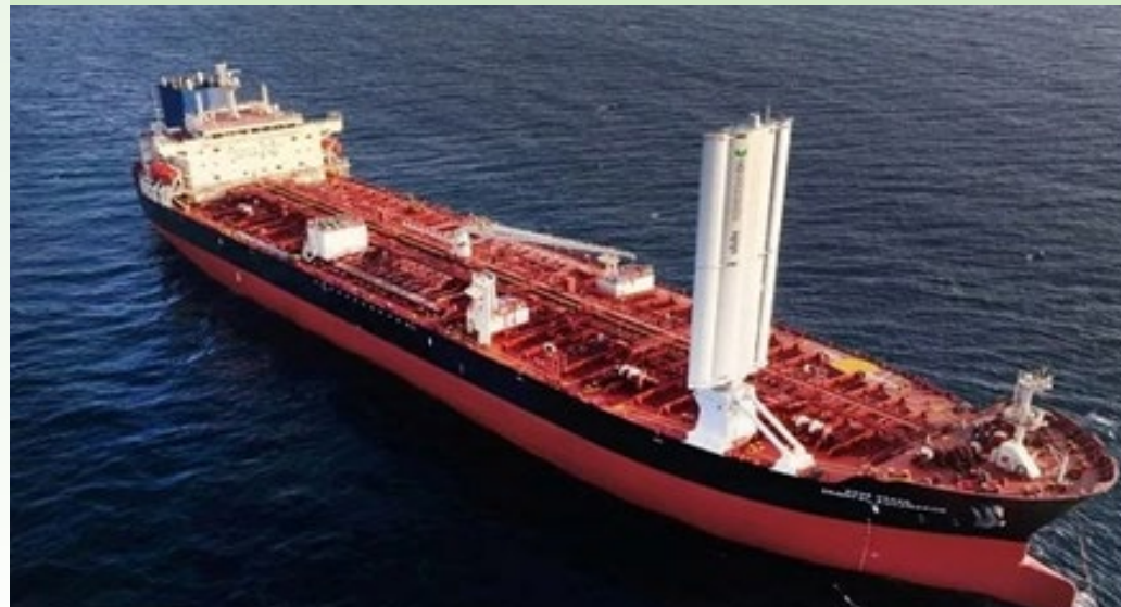
The Oriental Aquamarine with its fuel-saving sail.
