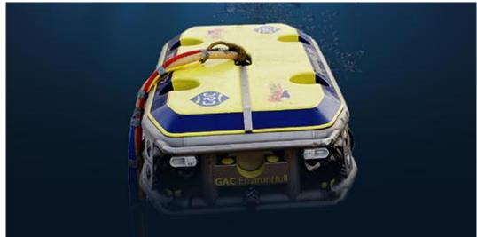
**Figure 7:** GAC EnvironHull's HullWiper hull-cleaning ROV. (source of photograph: GAC website: <u>www.gac.com/gacen/service.aspx?id=59651</u>).
