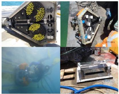
Figure 6: Franmarine Underwater Services' Envirocart cleaner. Top left: fitted with rotating brushes. Top right: fitted with rotating blades for contactless cleaning (blades are obscured to protect commercial confidentiality). Bottom right: "Magic box" for cleaning anodes and other projections. Bottom left: Envirocart in use (source of photographs: Franmarine Underwater Services' website, www.gageroadsdiving.com.au/projects/envirocart/).
