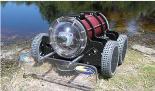
Figure 4: The US ONR's Hull BUG robotic cleaner. The version shown does not include the fluorometric sensor for detecting biofouling (source of photograph: ONR website, <u>www.onr.navy.mil/Media-Center/Fact-Sheets/Robotic-Hull-Bio-mimetic-Underwater-Grooming.aspx</u>).
