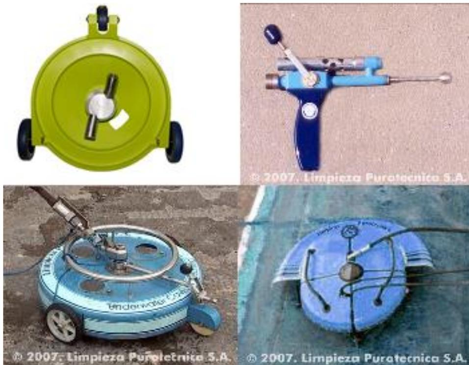
**Figure 8: Examples of cavitation-jet cleaning equipment.**
