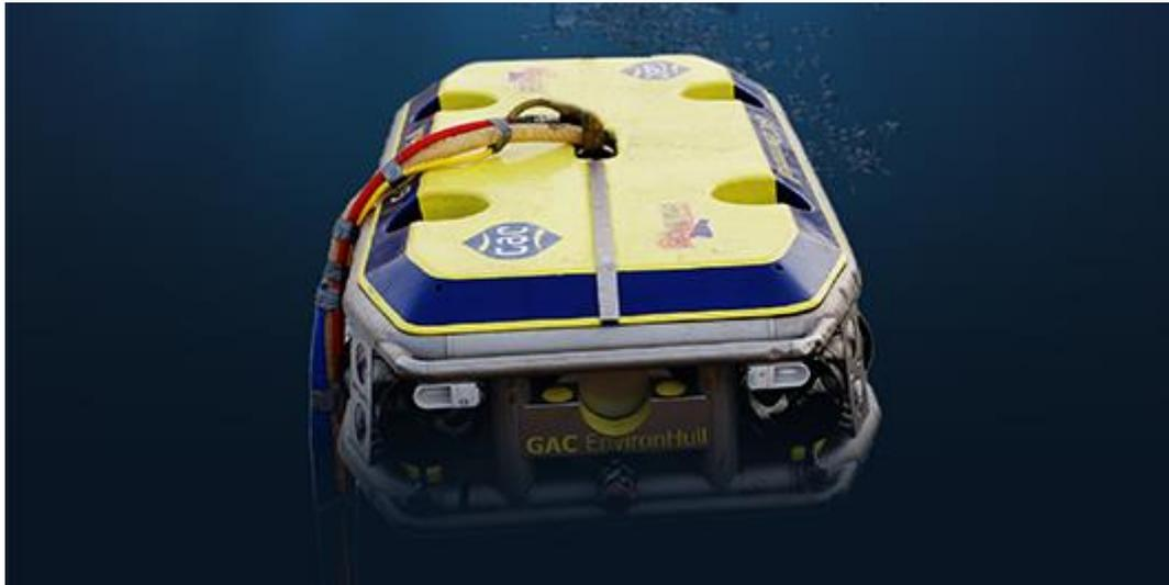
**Figure 7: GAC EnvironHull's HullWiper hull-cleaning ROV.**
