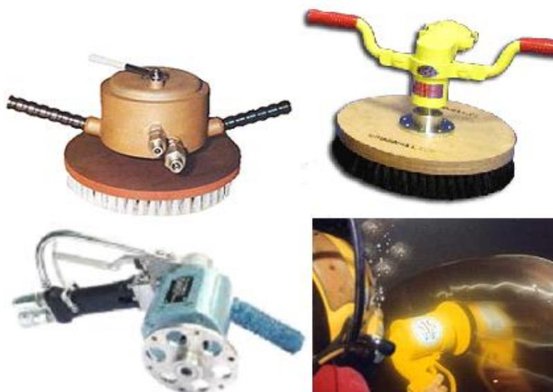
**Figure 1: Examples of brush- or pad-based hand tools for hull and propeller cleaning.**
