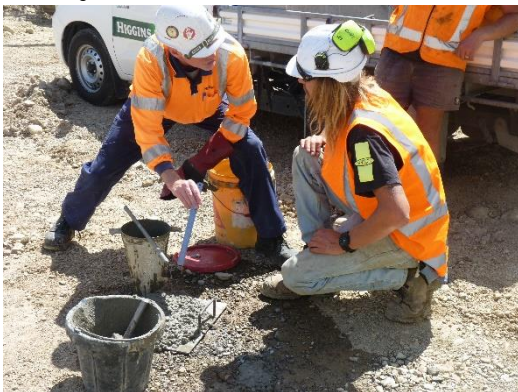
Contractors test the consistency of the concrete before pouring anchor piles.
