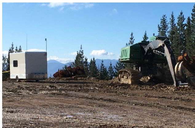
Purpose-built operator cabin and the tele-operated John Deere feller-buncher
