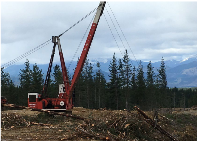
A yarder in action, showing the skyline and yarding carriage holding logs (the Skyshifter isn't installed on this yarder)
