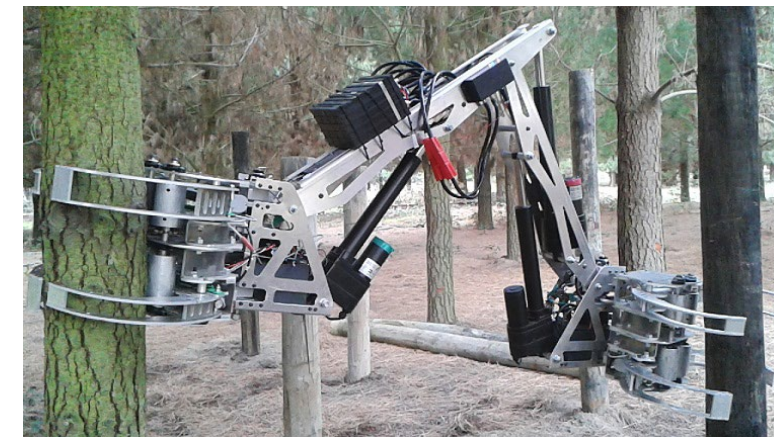
Prototype tree-to-tree robotic felling machine
