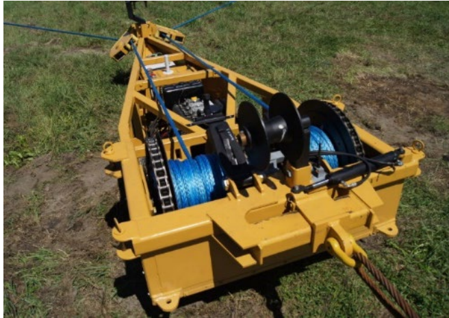
The beta prototype Skyshifter twin-winch tail-hold carriage
