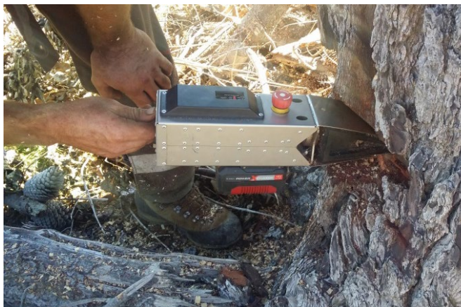
The remote-controlled powered felling wedge
