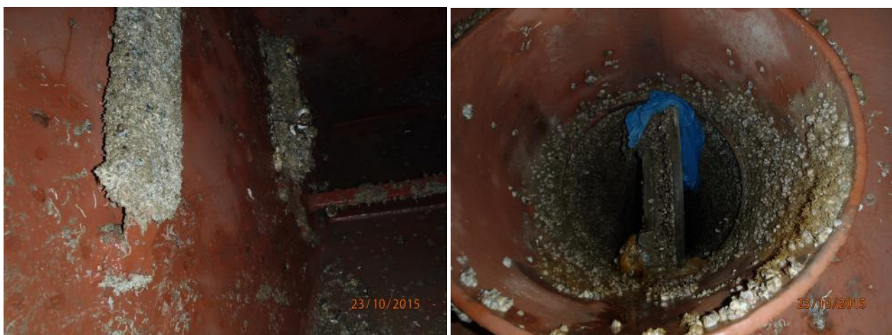
Figure 56. Biofouling on anodes and inside the intake of the same sea chest as in the previous figure.
