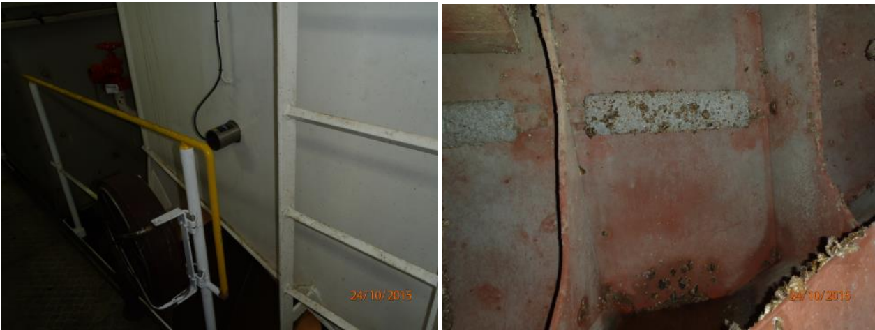
Figure 70. Ultrasound generator attached to the outside of the sea chest and corresponding location inside the sea chest.
