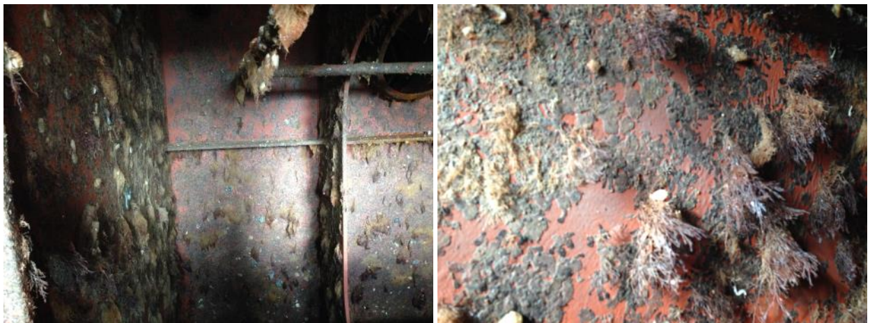
Figure 32. CDP2-coated sea chest at 15 months with walls almost completely covered by bryozoans and other macrofouling.
