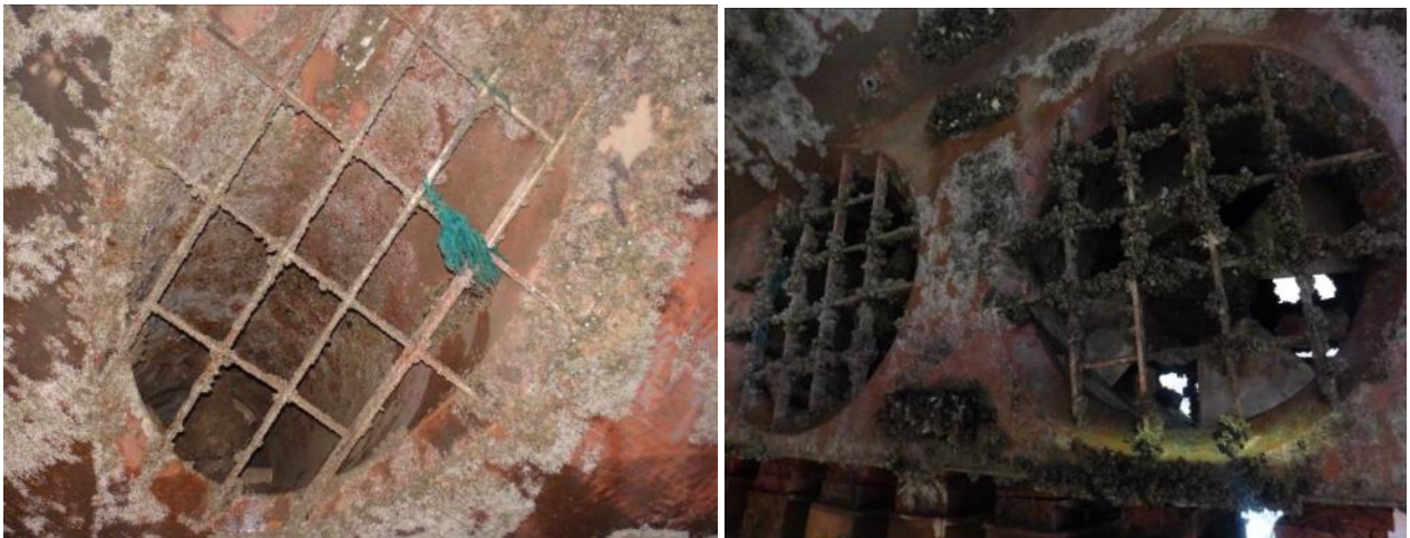
Figure 47. CDP painted thruster tunnels and tunnel grates after 40 months showing extensive macrofouling establishment on grate bars and tunnel walls.
