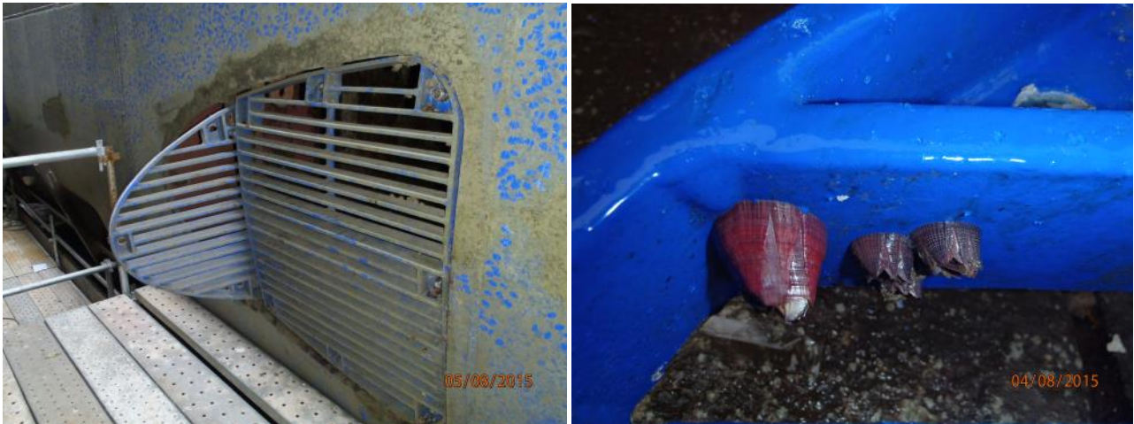
Figure 24. FRC-coated sea chest intake grate at 36 months with only a few barnacles on paint imperfections.
