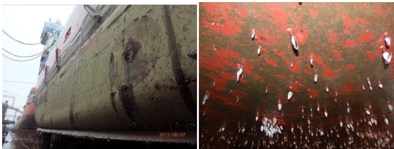
Figure 15. Acorn and goose barnacle and slime fouling on SPC on sides and flats of one vessel at 40 months.
