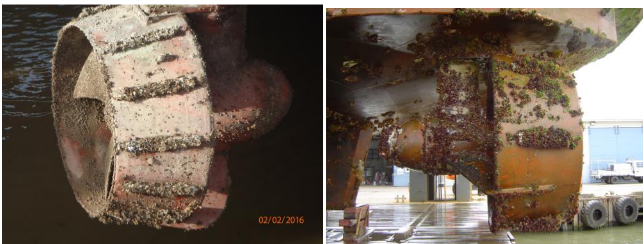
Figure 40. CDP-coated Schottel propulsion units on two vessels after 13 (left) and 36 (right) months service, both with scattered macrofouling on paint surfaces and substantial fouling on anodes and paint imperfections.
