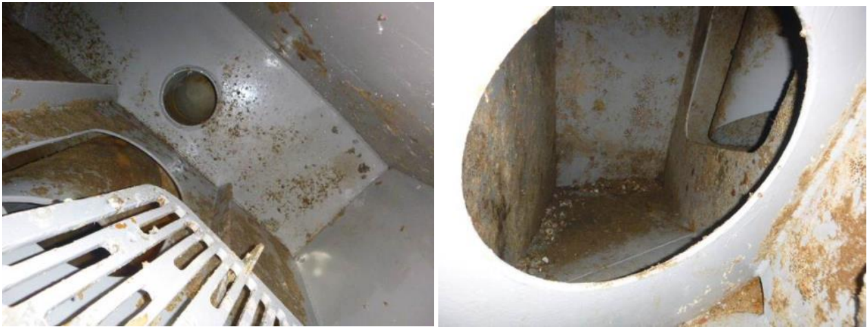
Figure 36. FRC-coated sea chest at 17 months showing up to 50 % coverage of walls by encrusting biofouling.
