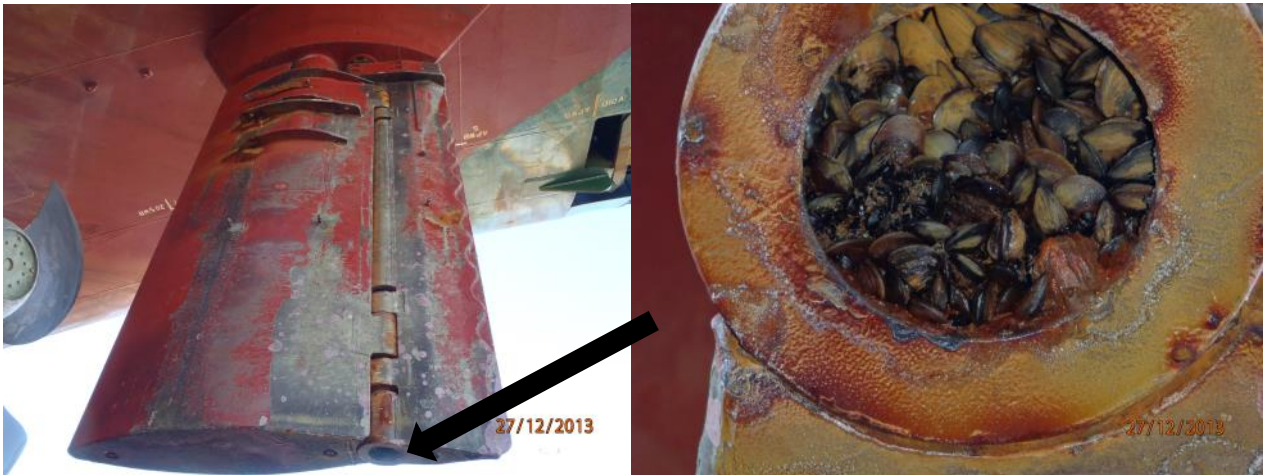
Figure 44. FRC-coated rudder at 24 months with little macrofouling on rudder surfaces but substantial mussel growth in the lower pintle recess (arrowed).
