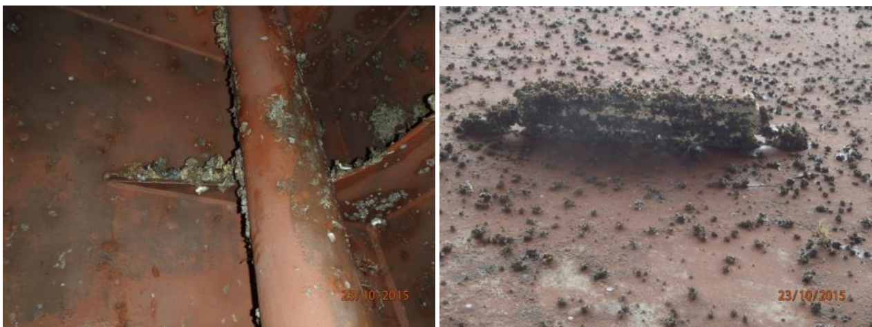
Figure 38. Vessel after 7 months in service with CDP1 coating performing better inside the sea chests than on the outer hull.
