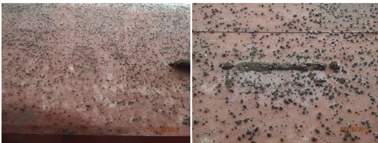
Figure 8. Barnacle fouling on CDP coating of one vessel at 7 months.
