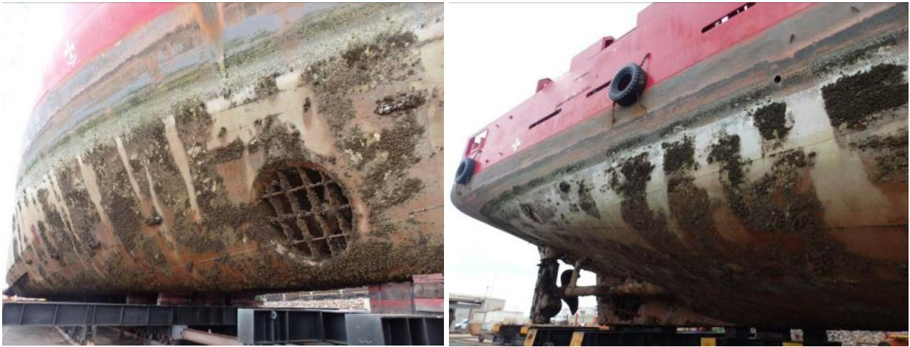
Figure 11. Patches of barnacle fouling on CDP coating on one vessel at 36 months.
