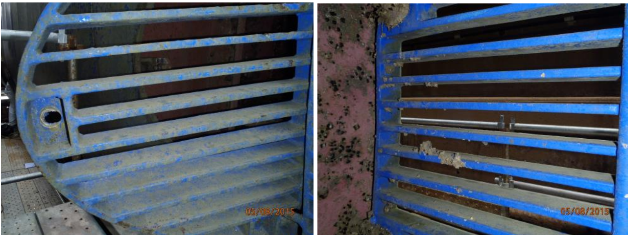
Figure 25. FRC-coated sea chest intake grate of same vessel as in previous figure showing bars almost free of macrofouling.
