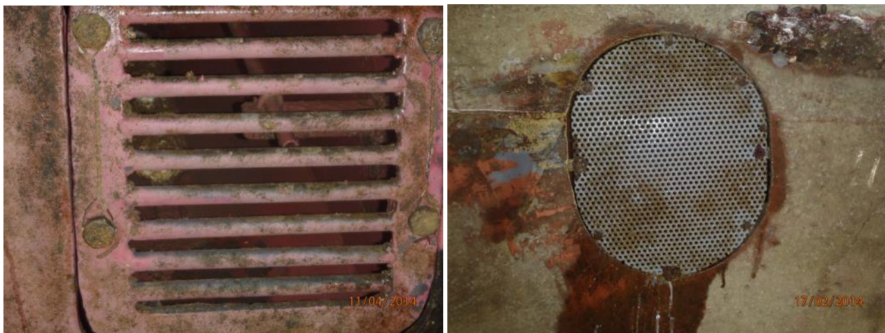
Figure 21. SPC- (left) and FRC (right) coated sea chest intake grates on two vessels with similar operational profiles, both with minimal macrofouling on the grates.
