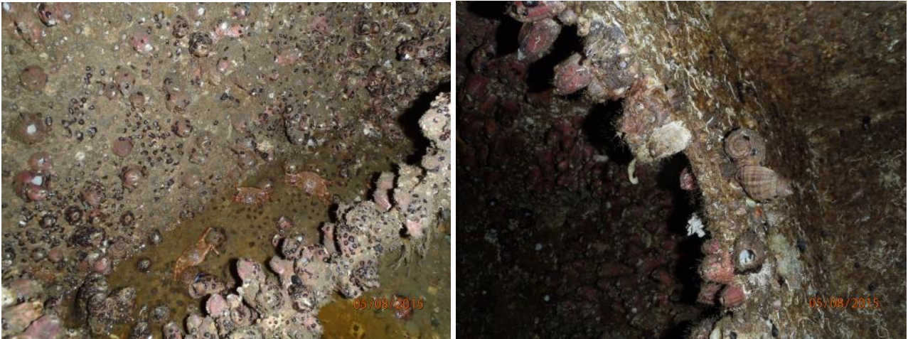
Figure 54. Tertiary stage biofouling, including crabs (left) and dog whelks (right) in the same sea chest as in Figure 52.
