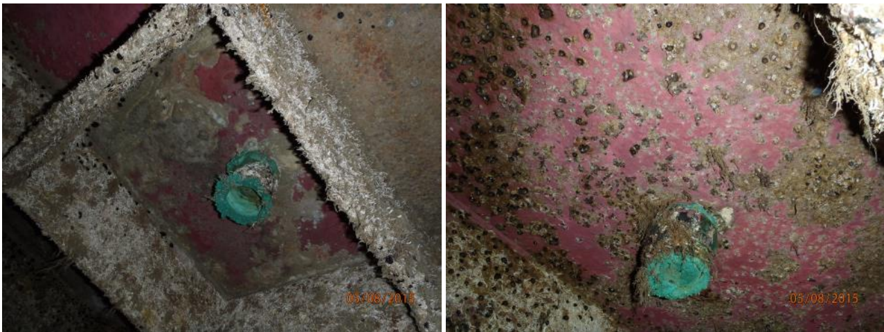
Figure 52. Depleted copper anodes inside a sea chest with a “hard” CDP coating after 36 months service, showing extensive macrofouling on the chest walls and projections.
