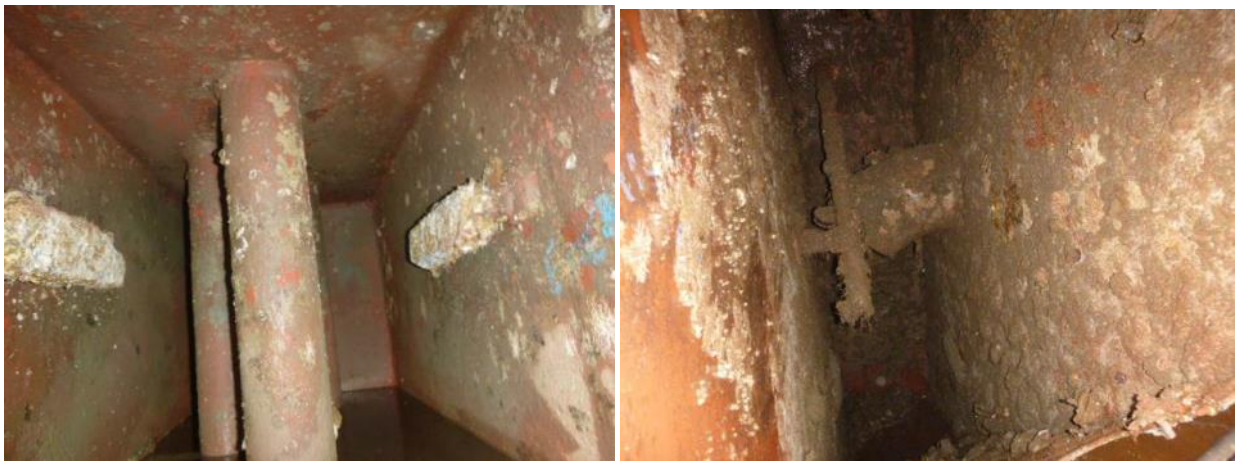
Figure 29. CDP1-coated sea chests on one vessel at 30 months showing extensive biofouling cover on walls and projections.
