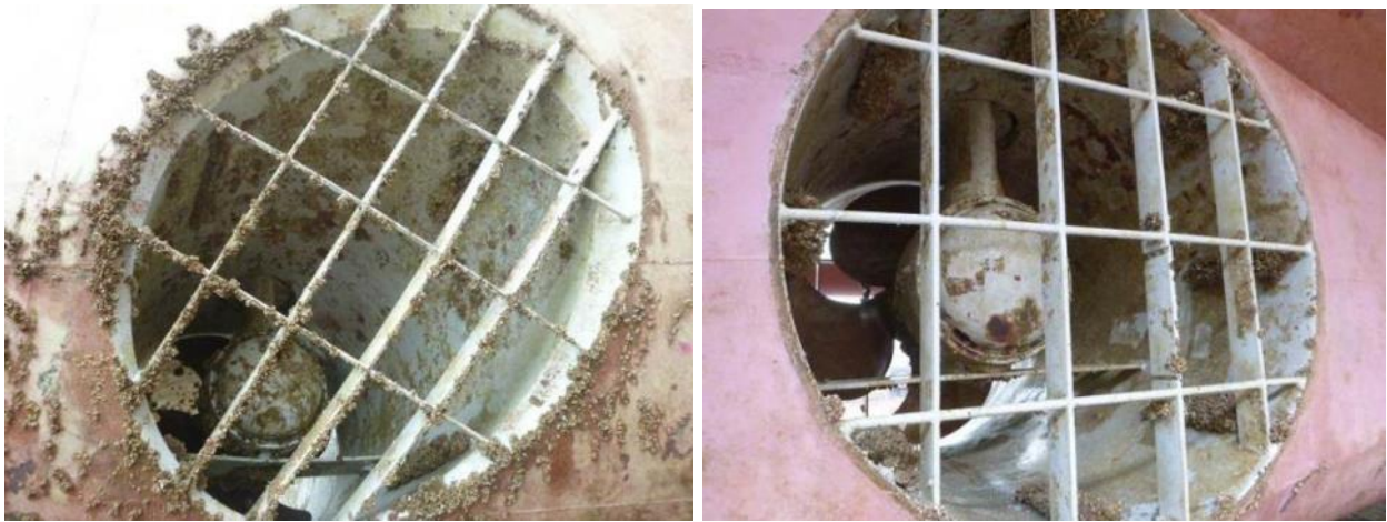
Figure 49. FRC-painted thruster tunnels and grates on one vessel after 17 months showing minimal to little macrofouling on grates.
