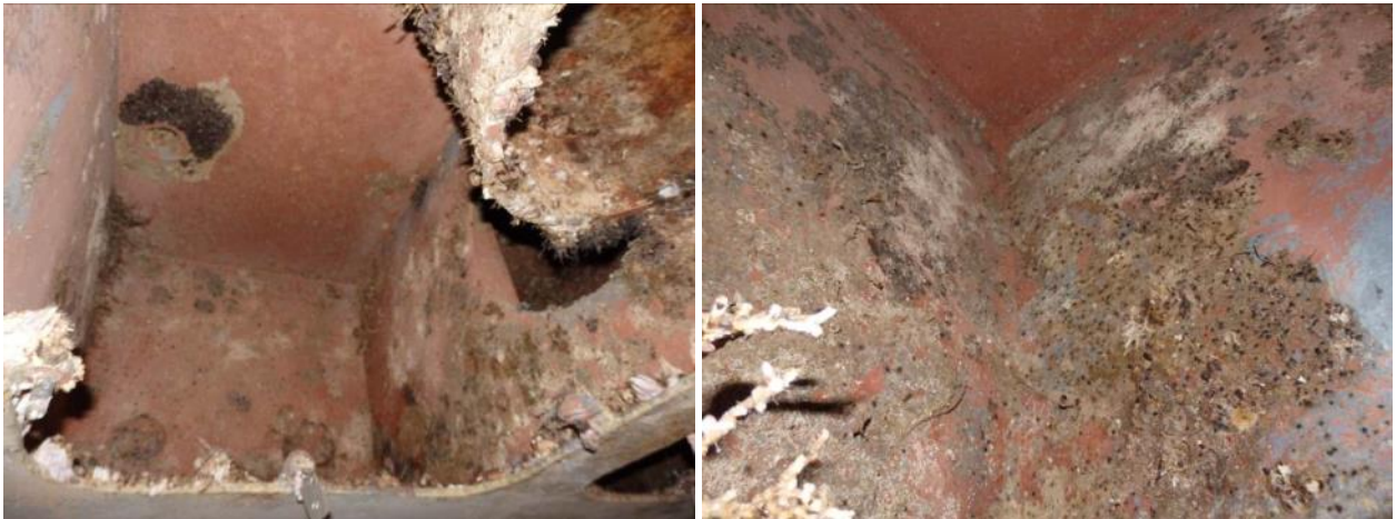
Figure 30. CDP1-coated sea chests on one vessel at 36 months with extensive fouling on chest walls.
