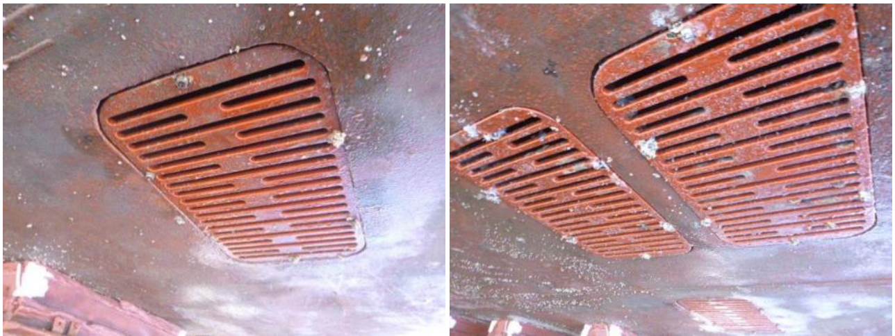
Figure 19. CDP-coated sea chest intake grate bars at 30 months with minimal macrofouling.
