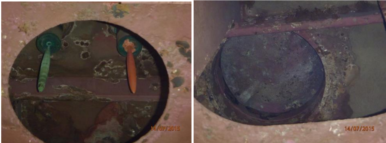
Figure 51. Copper and aluminium MGPS anodes inside a sea chest with a “soft” SPC coating after 24 months service with low abundance of macrofouling on the chest walls.
