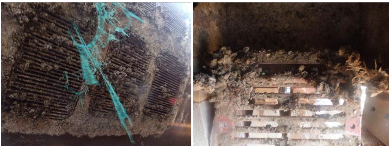
Figure 20. CDP-coated sea chest intake grate bars at 40 months with high abundance of macrofouling on, between and under grate bars.
