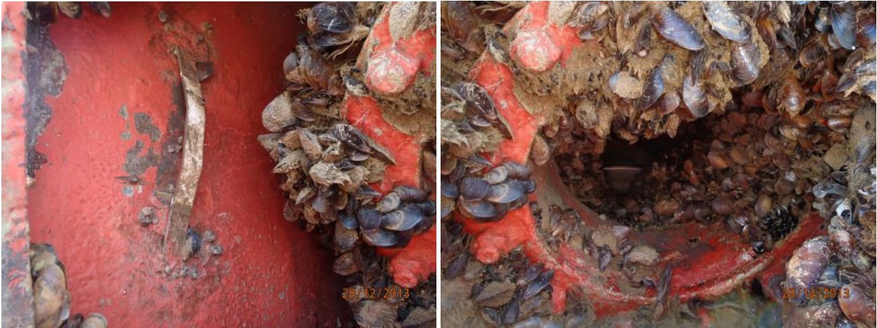
Figure 28. CDP1-coated sea chest on one vessel at 24 months showing minimal macrofouling on the chest wall (left) and heavy fouling on projections (left and right).
