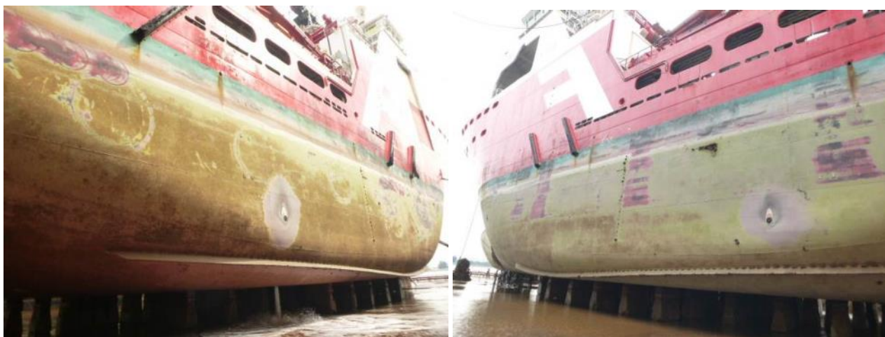
Figure 14. Slime on SPC on vertical sides of one vessel at 17 months.
