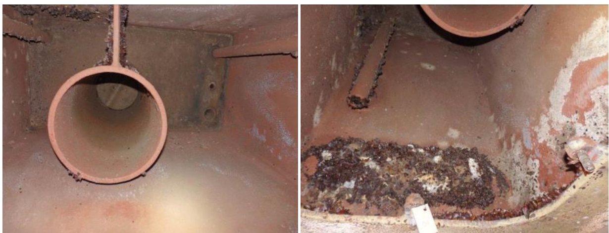
Figure 31. Other CDP1-coated sea chests on the same vessel as in Figure 30, but macrofouling mostly restricted to projections.
