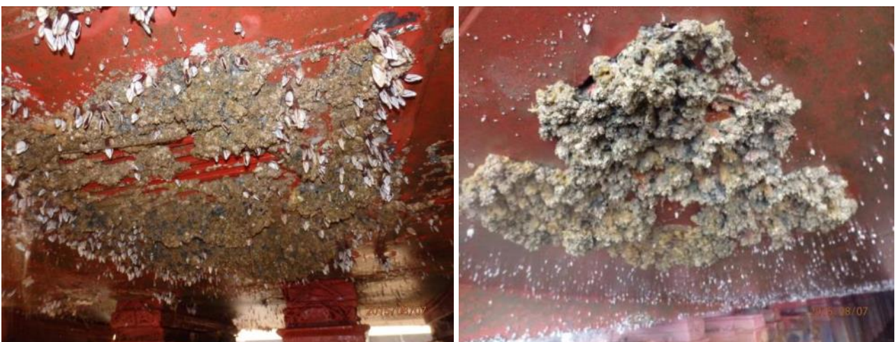
Figure 26. FRC-coated sea chest intake grates on a vessel at 40 months with apparent extensive macrofouling on the grates. This was determined to be overgrowth from fouling establishing on unpainted attachment bolts and edge damage.
