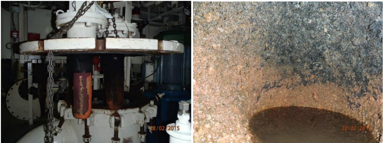
Figure 67. The low intake strainer box on the same vessel as Figure 66 with no viable fouling present.
