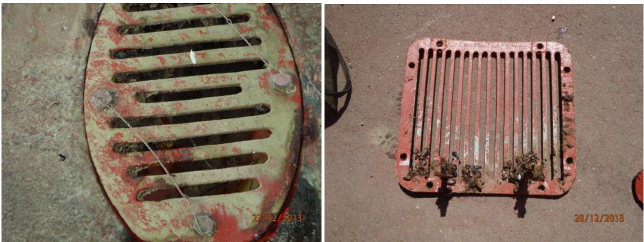
Figure 18. CDP-coated sea chest intake grate bars at 24 months with low abundance of macrofouling between bars.
