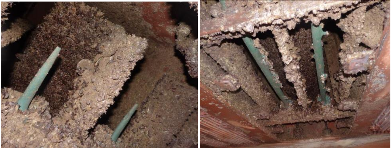
Figure 62. Box cooler with copper anodic MGPS after 40 months, with extensive macrofouling on all surfaces except for the anodes themselves.
