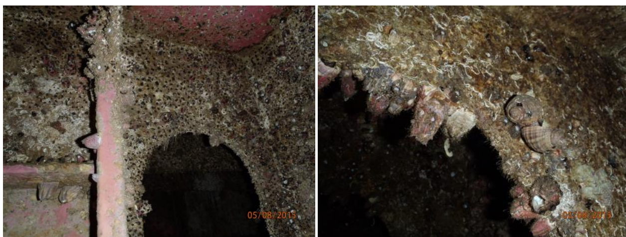
Figure 35. SPC2-coated sea chest at 36 months with extensive coverage of macrofouling on walls and tertiary stage 7 biofouling on projections.
