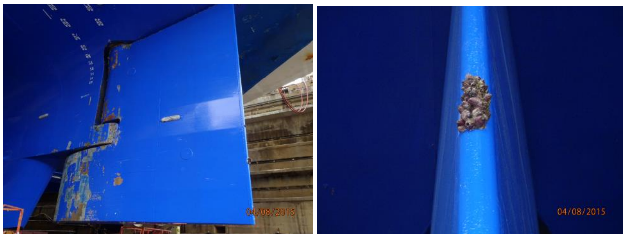
Figure 43. FRC-coated rudder at 36 months with macrofouling confined to areas of paint damage.
