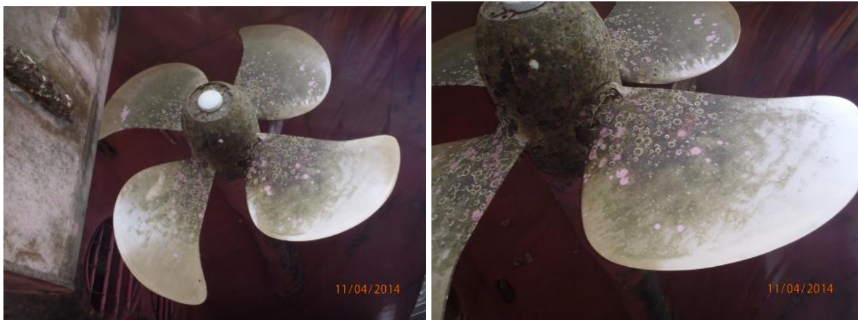
Figure 45. Unpainted propeller with low-profile macrofouling on the hub and inner surfaces of blades.
