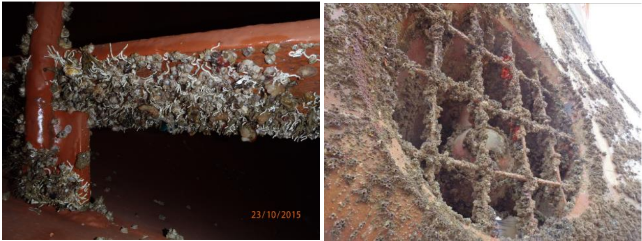
Figure 48. CDP painted thruster tunnel grates on two vessels after 7 (left) and 36 (right) months in service showing substantial macrofouling establishment on grate bars.
