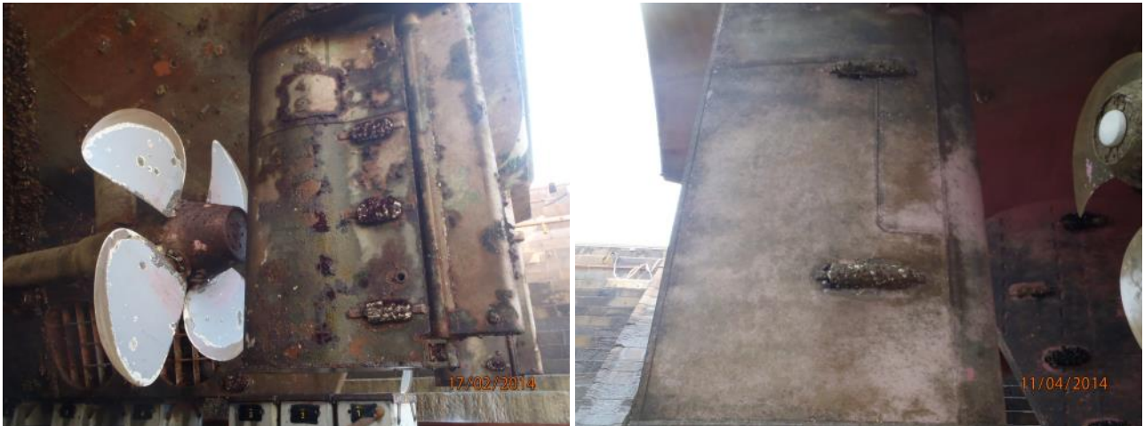
Figure 41. CDP- (left) and SPC- (right) coated rudders on two vessels with similar operating profiles showing less macrofouling on the SPC.
