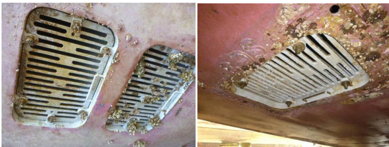
Figure 22. FRC coated sea chest intake grates on one vessel at 17 months with overall minimal macrofouling on and between bars.
