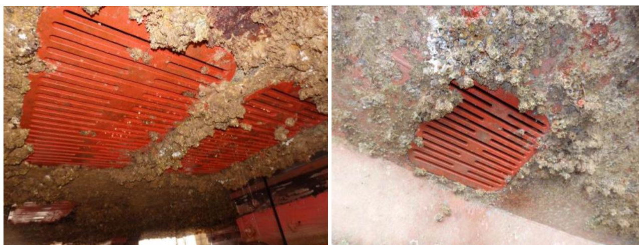
Figure 23. FRC coated sea chest intake grates at 36 months with minimal macrofouling despite extensive fouling on adjacent hull surfaces.
