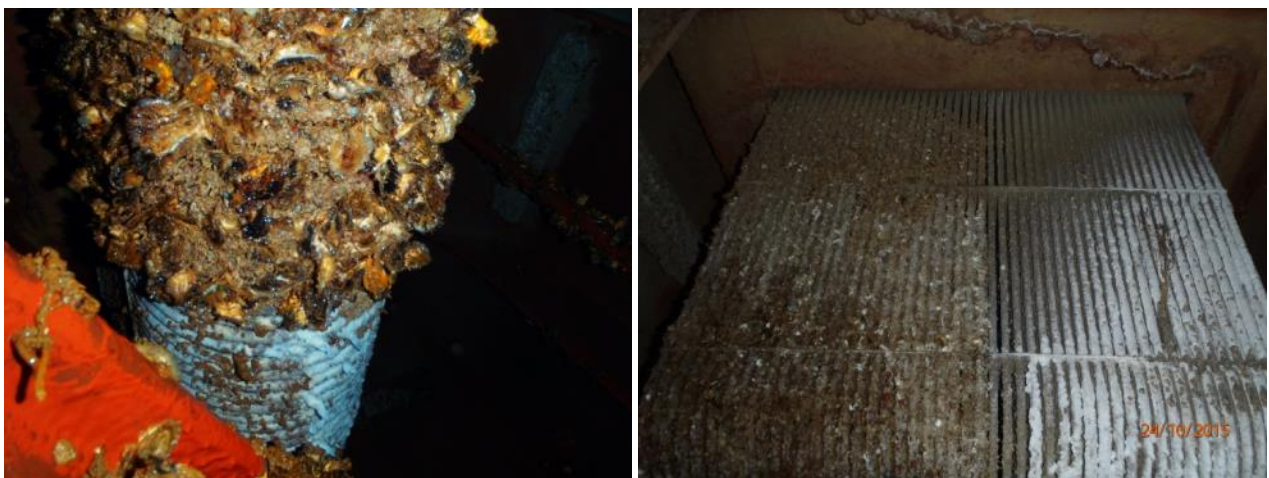
Figure 60. Box cooler after 7 months operation with substantial macrofouling on “cool” half, and only inorganic chalk on the “hot” half.
