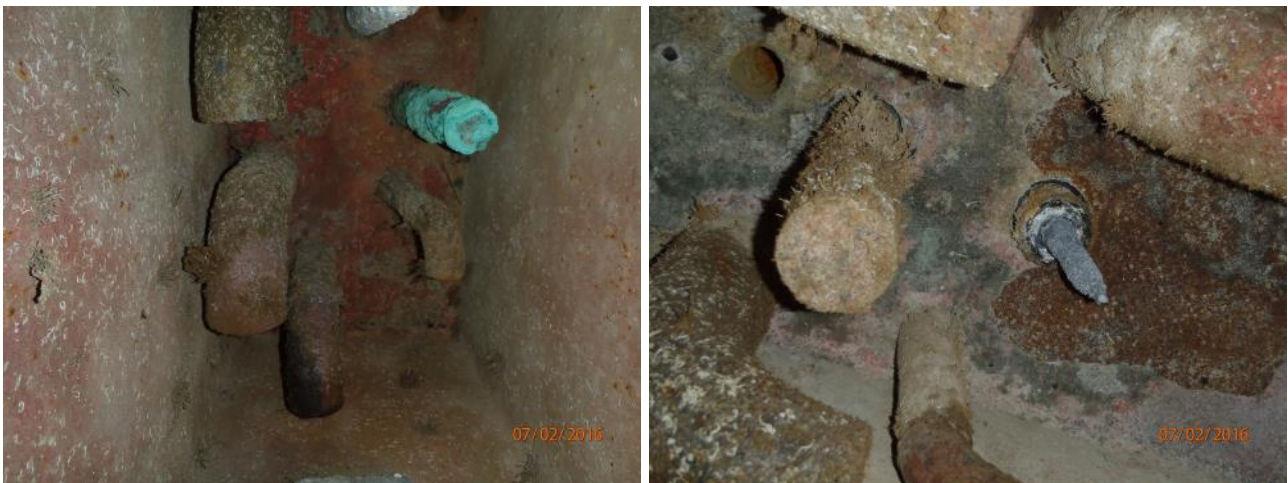
Figure 58. MGPS anodes inside sea chest of a Southern Ocean fishing vessel with tubeworms on chest walls and hydroids and tubeworms on projections.
