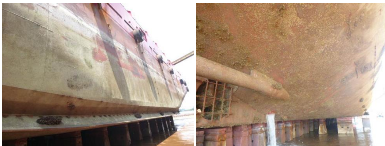
Figure 10. Extensive secondary 6 fouling on CDP coating on one vessel at 30 months.
