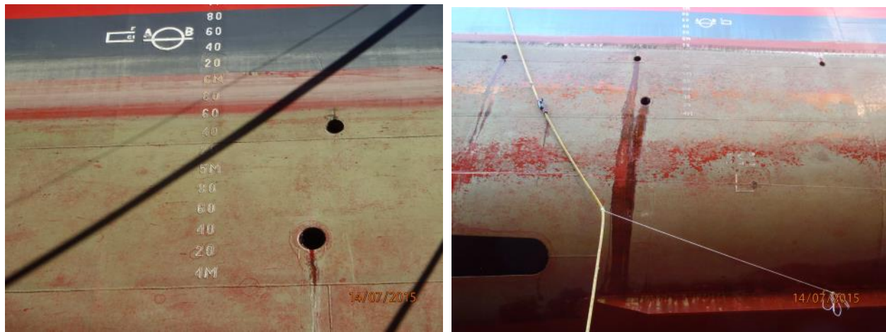
Figure 5. FRC on boottop and vertical sides at 23 months with only slime (primary biofouling).
