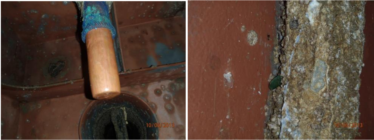
Figure 57. Sea chest on the same vessel as in the previous figures, but at an earlier docking. Note the growth on inner walls of the unpainted intake pipe and under the anode (including Asian green mussel ( Perna viridis )).
