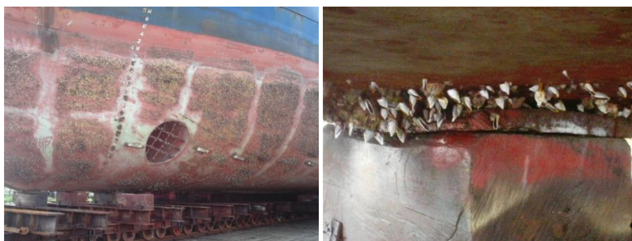
Figure 9. Scattered patches of goose and acorn barnacle fouling on CDP coating on one vessel at 15 months.
