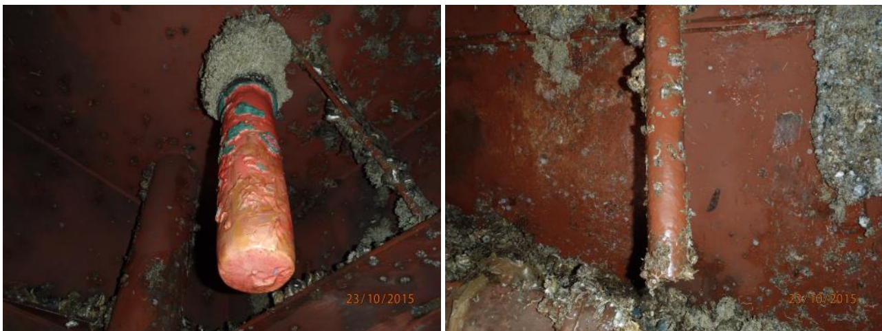
Figure 55. Biofouling in a sea chest fitted with a copper anodic MGPS after 7 months service showing a tubeworm collar around the base of an anode (left) and secondary fouling on an anode and projections (right).
