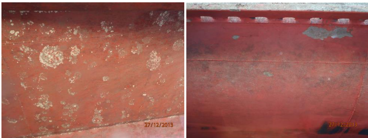
Figure 13. FRC (left) and CDP (right) on flats of same vessel at 24 months. Scattered encrusting bryozoan colonies were present on the FRC.
