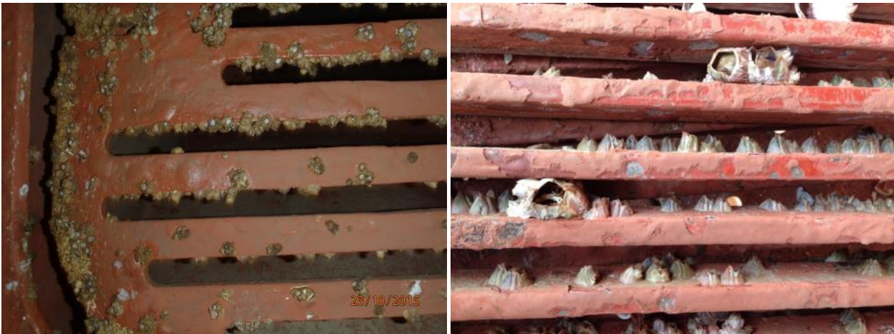
Figure 17. CDP-coated sea chest intake grates on vessels after 7 (left) and 15 (right) months service with acorn barnacles predominantly clustered along grate edges and between bars.
