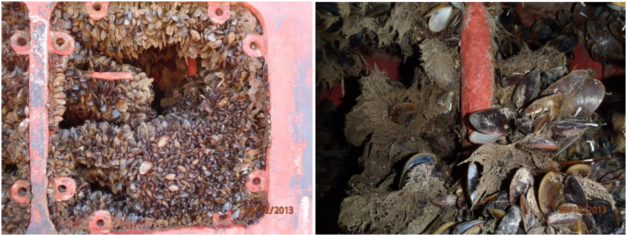
Figure 69. Mussels in the chemically dosed sea chest, including around the dosing pipe.
