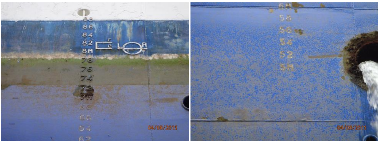
Figure 7. SPC boottop and FRC on vertical sides of the same vessel at 36 months. Green algal band along the boottop; only slime on the vertical sides.
