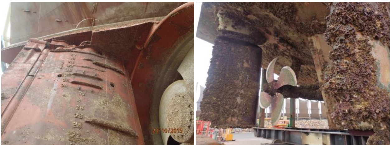
Figure 39. CDP-coated rudders on vessels after 7 (left) and 40 (right) months service showing the development of biofouling over time.
