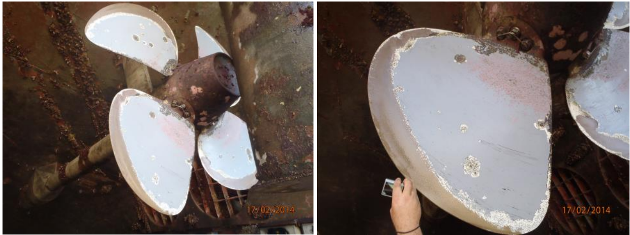
Figure 46. FRC-painted propeller on a vessel with a similar operating profile to that in Figure 43 showing absence of comparable macrofouling on the blades.
