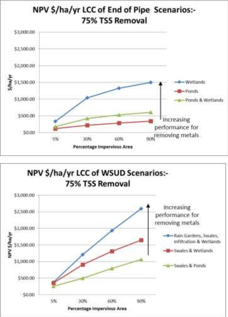
**Figure 3-12: Examples of costing models developed for traditional (upper plot) and WSD (lower plot) forms of stormwater treatment. After Ira (2011; 2015a).**
