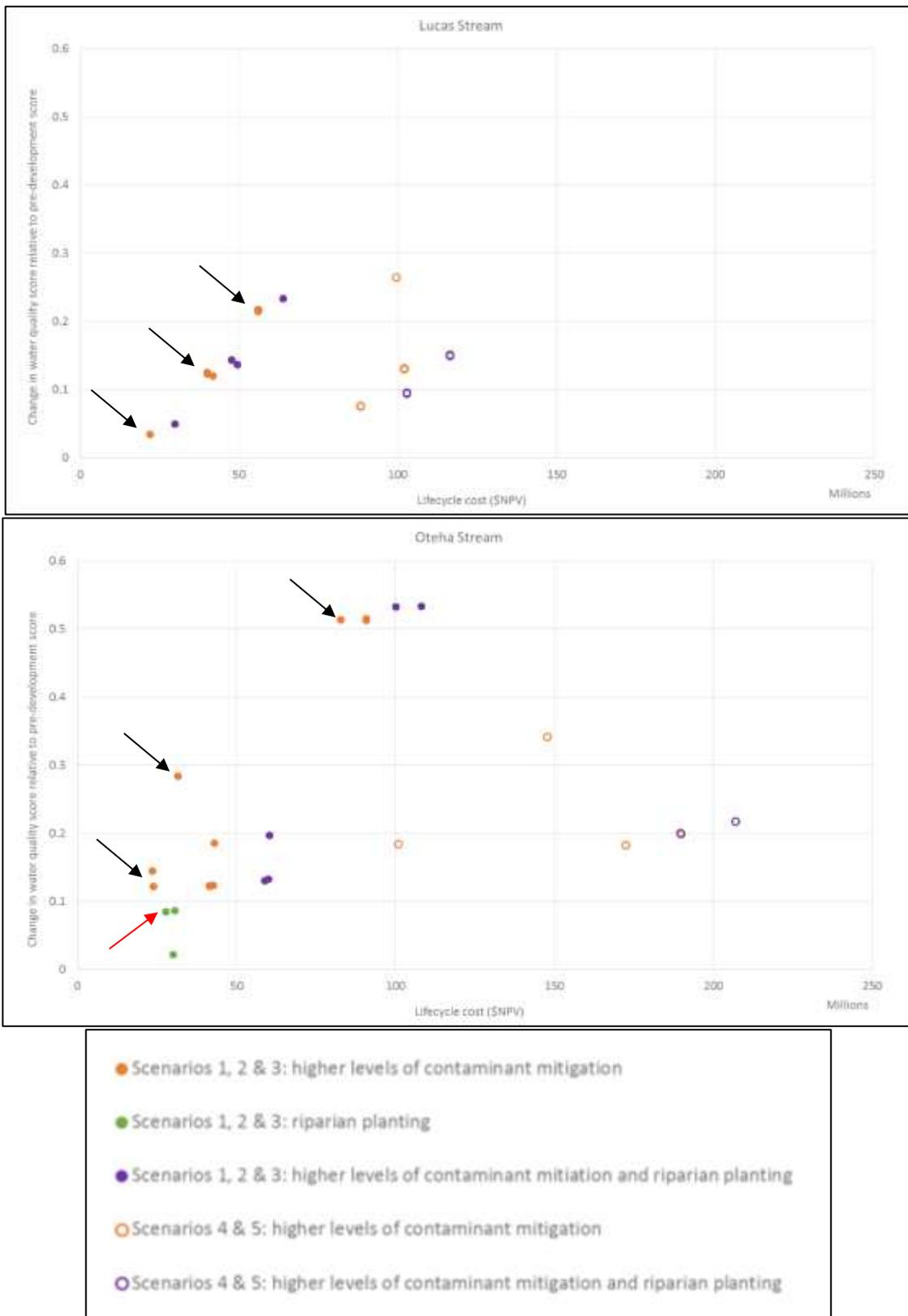
**Figure 3-15: Relationship between the costs of mitigation and the change in the water quality indicator score for scenarios which result in an improvement relative to the pre-development score, Lucas Stream (upper) and Oteha Stream (lower).** Costs are estimated over 50-years using a discount rate of 8%. Arrows indicate examples referred to in the text.
