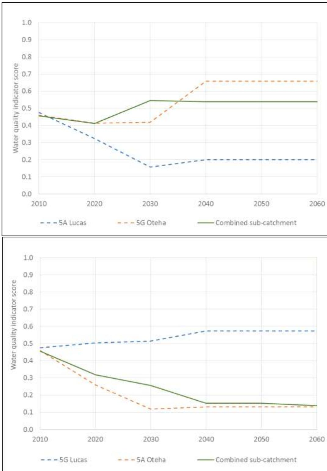
**Figure 3-11: Predicted water quality indicator scores for selected higher density greenfield development scenarios: Lucas Stream, Oteha Stream and their combined sub-catchment.** The scenario represented in the upper plot involves *status quo* contaminant controls in the Lucas Stream sub-catchment (5A) and a high level of contaminant controls with extensive riparian planting in the Oteha Stream (5G). The scenario represented in the lower plot represents the reverse situation.
