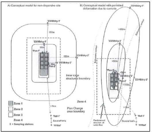
Figure 3: Conceptual model for Zonal approach to monitoring. Source: (Keeley 2012)
