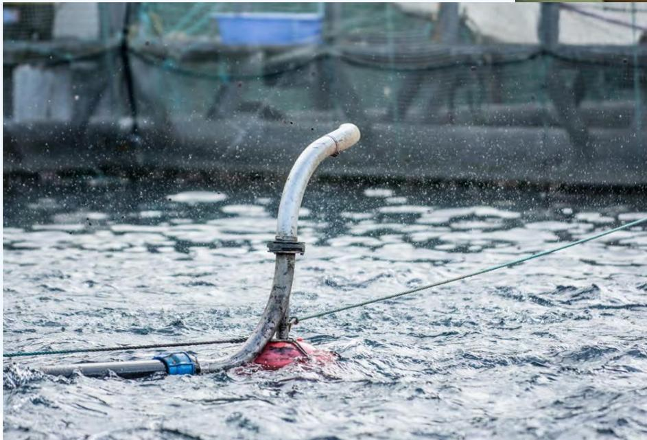
**Roto feeder - spreads feed
