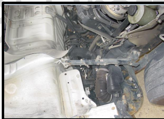
Clean the radiator and surrounding area removing all contamination. An air gun or vacuum can help remove contamination from crevices around motor.
