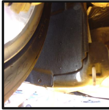
Thoroughly check mudguards, tyres and wheel arches. Water blast if required.
