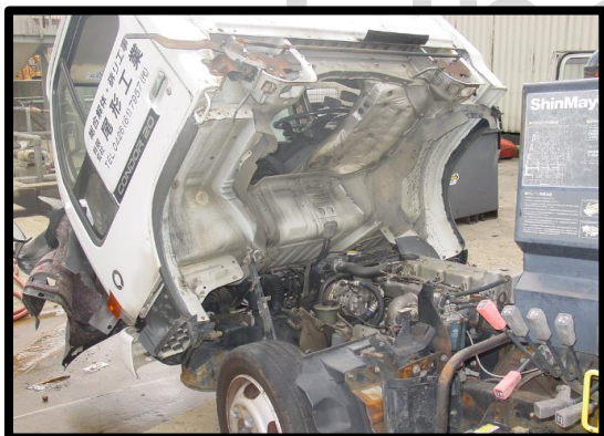
Clean the radiator and surrounding area removing all contamination. An air gun or vacuum can help remove contamination from crevices around motor.
