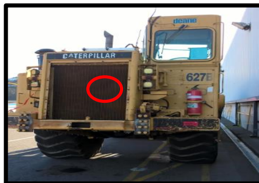
Inspect and clean filters, grates and grilles for contamination caught within. Where possible remove these parts and leave off during importation.
