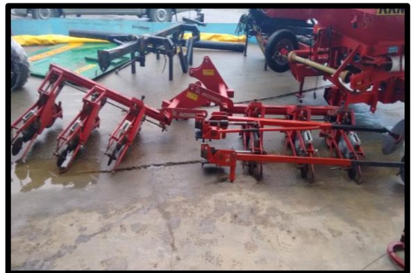
Clean all areas that have had contact with plant material and soil. Check all component hinges. Shine a bright light up any metal structures that are hollow.
