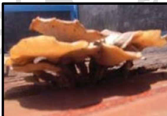
If fungal structures (fruiting body) are present, wood will need to be removed or treated.
