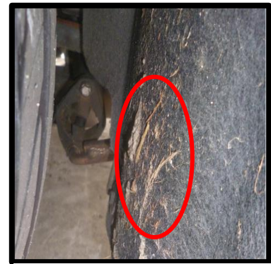
If mud guards are covered in felt, thorough scrubbing or water blasting will be needed.
