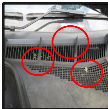
Remove contamination around bonnet and grilles.
