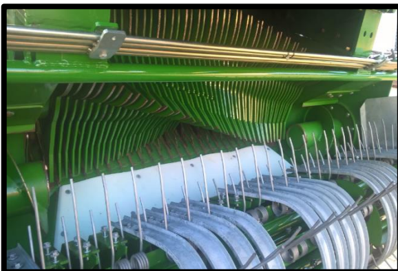
Remove all plant material caught in the comb/teeth. Dismantle and clean all internal compartments.
