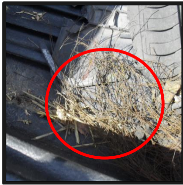
Remove any plant material or pooled water from the vehicle.
