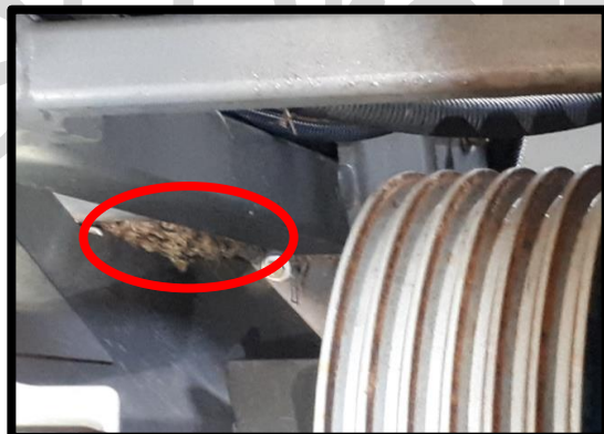
Use a bright light to inspect what you can of the vehicle underside such as plant material or soil (circled). A high pressured water hose can help clean what you may not be able to see.
