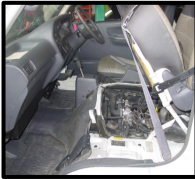
If motor is accessible from cab, use a vacuum or air gun to remove any contamination.
