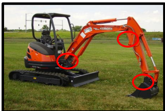
Inspect the entire boom area. Clean all hinges, swivel points and between the entire lengths of cable bundles.
