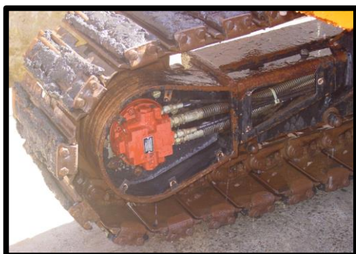
Waterblast all track pads, track chains and other cavities to ensure they are free of soil and other contaminants. Deconstruct as much as possible panels and plates off during importation. This includes non-affixed panels, rock guards and motor covers.
