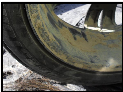
Water blast tyres and mud guards. A light road film is ok but anything more than this is not considered clean
