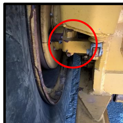
Inspect all wheel arches/joining for contamination, especially insect or spider egg masses.
