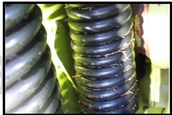
Remove all plant material trapped between small crevices and cables.
