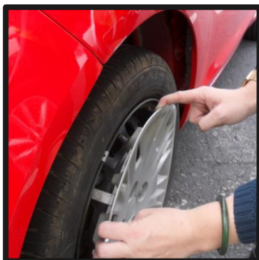
Remove hubcap, check for contamination, especially eggs masses around tyre and wheel area.
