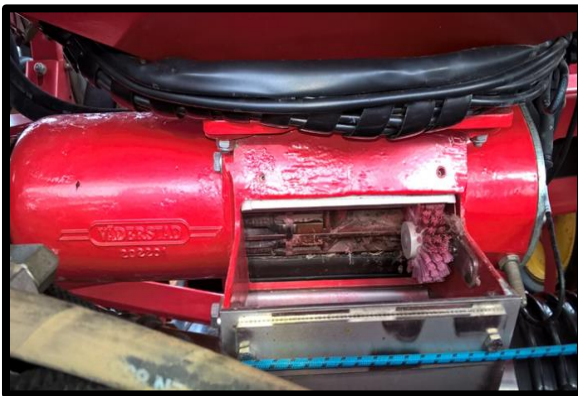
Open all possible compartments for cleaning. Use high pressure air or a vacuum with an adaptable head where required.
