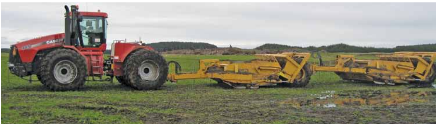
Land reshaping guided by high accuracy GPS will avoid crop loss in high drought and low wet areas – yield maximised for given energy and nutrient inputs.
