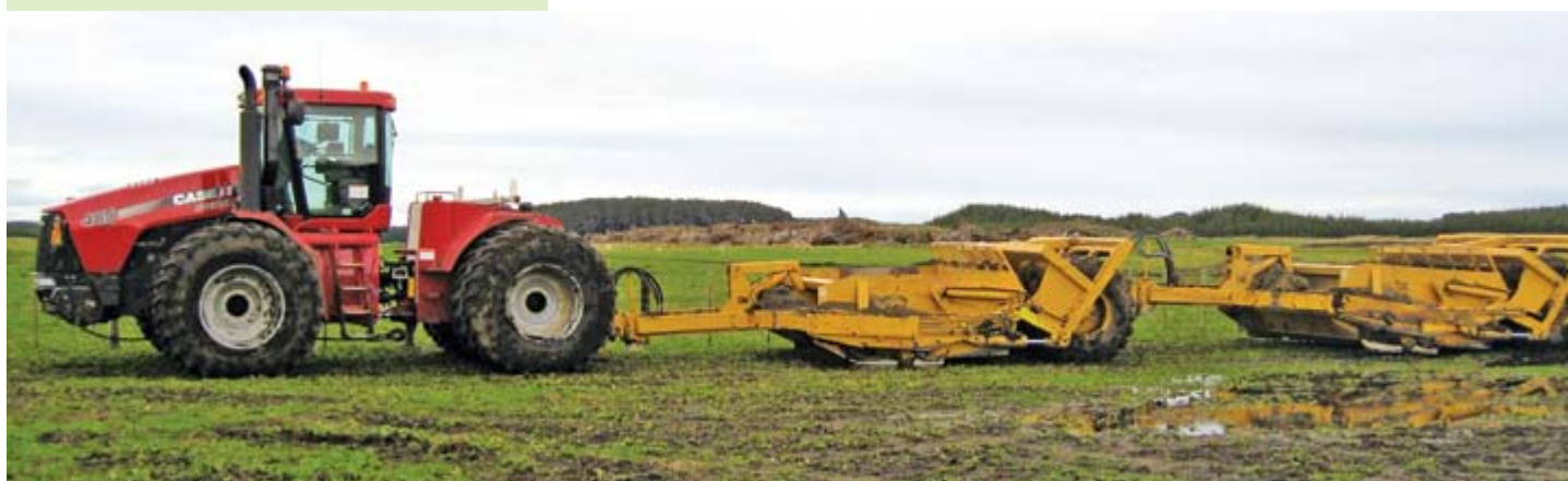
Land reshaping guided by high accuracy GPS will avoid crop loss in high drought and low wet areas – yield maximised for given energy and nutrient inputs.
