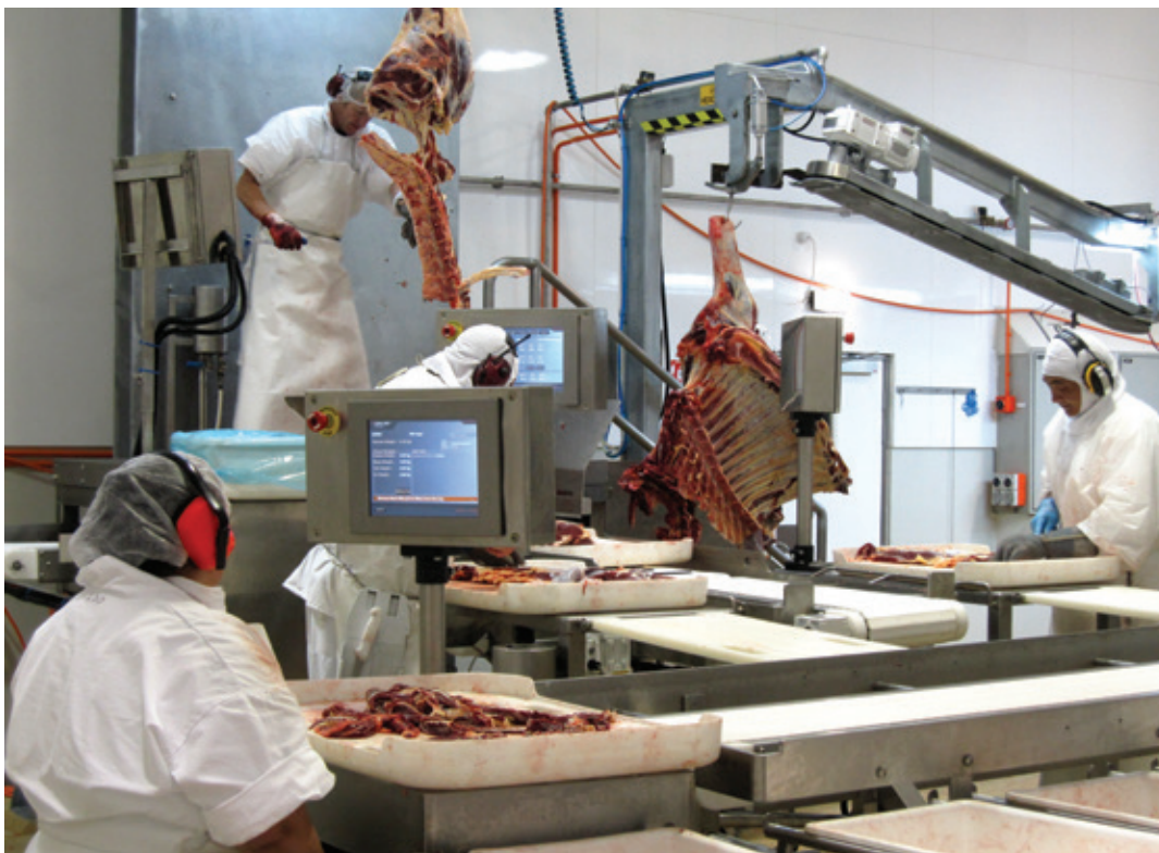
An experimental beef boning station at Finegand using RFID tags embedded in plastic trays for yield measurement.
