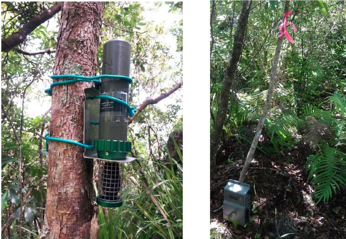
**Figure 2.3:** Representative examples of the field deployment of DOC ARU (left-hand image) and Song Meter 2+ (right-hand image) passive acoustic devices on Little Barrier and Great Barrier Islands.
