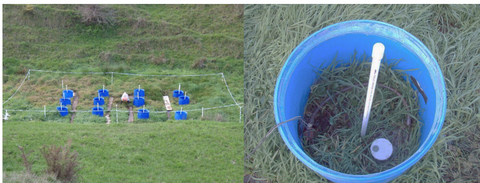
Figure 7. A. Array of 12 mesocosms in the headwater wetland. B. Inside view of mesocosm showing pump to circulate water, piezometer to sample subsurface water and chamber to collect emitted nitrous oxide.
