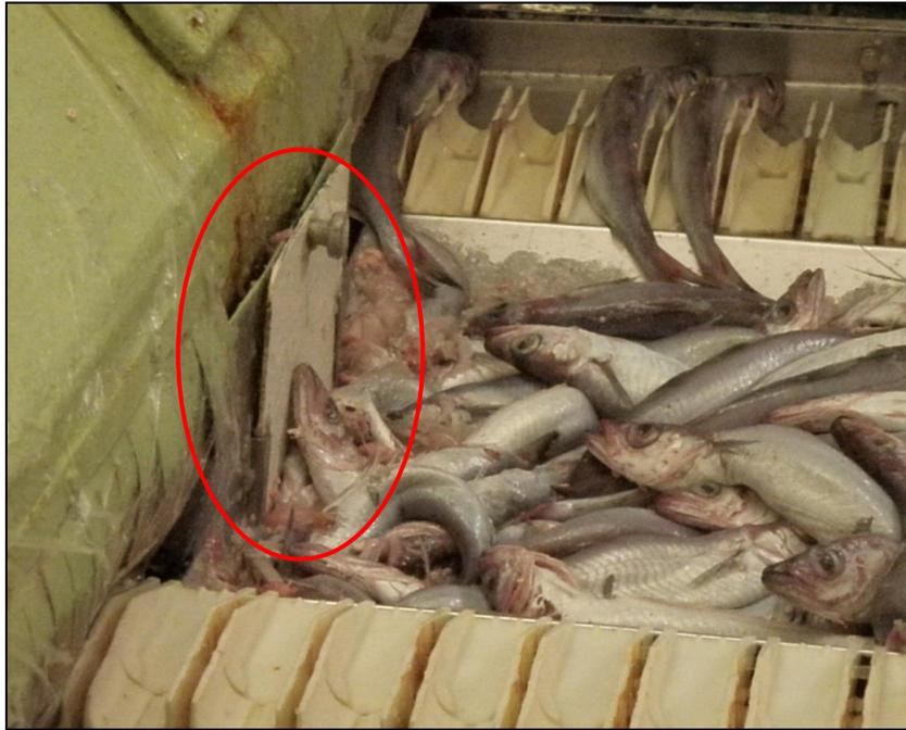
Figure 11 - Sliding lid provides ease of access to divert fish to IRA offal.
