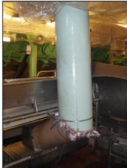
Figure 10c - Chute from trawl deck direct to meal auger.
