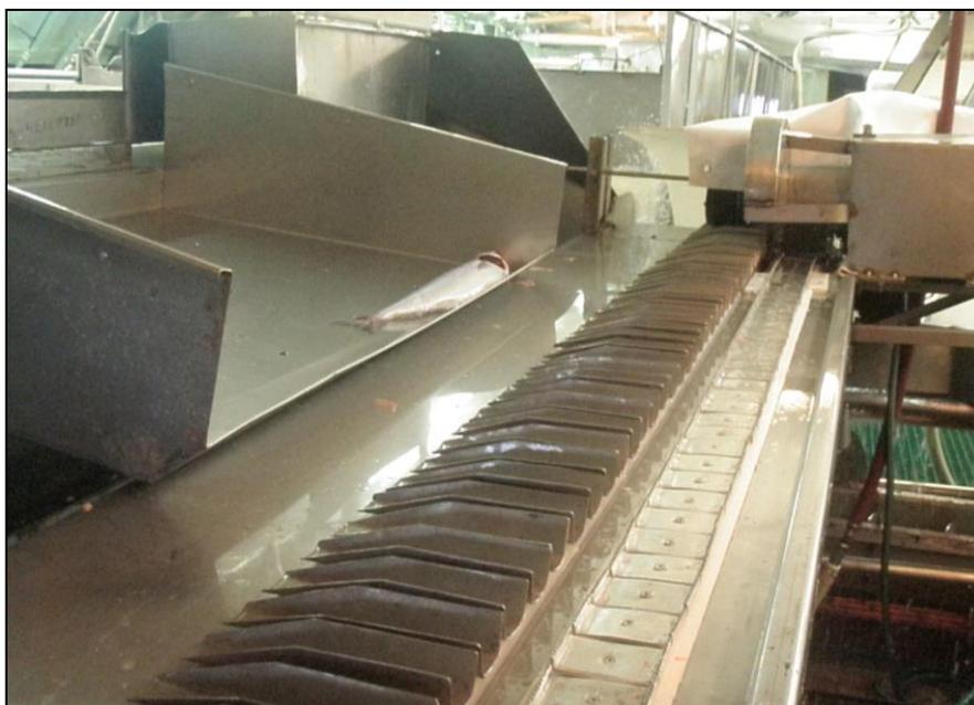
Figure 5 – Conveyor with fish body trays for feeding fish into circular saw on vessel 4.
