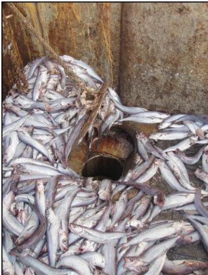
Figure 10b - chute from trawl deck hopper direct to meal auger (in some instances via main sorting hopper)
