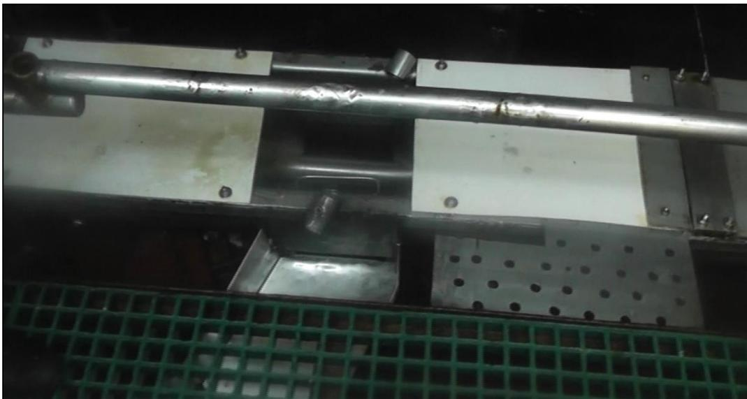
Figure 4 – Shows chute from meal auger with removable plate.
