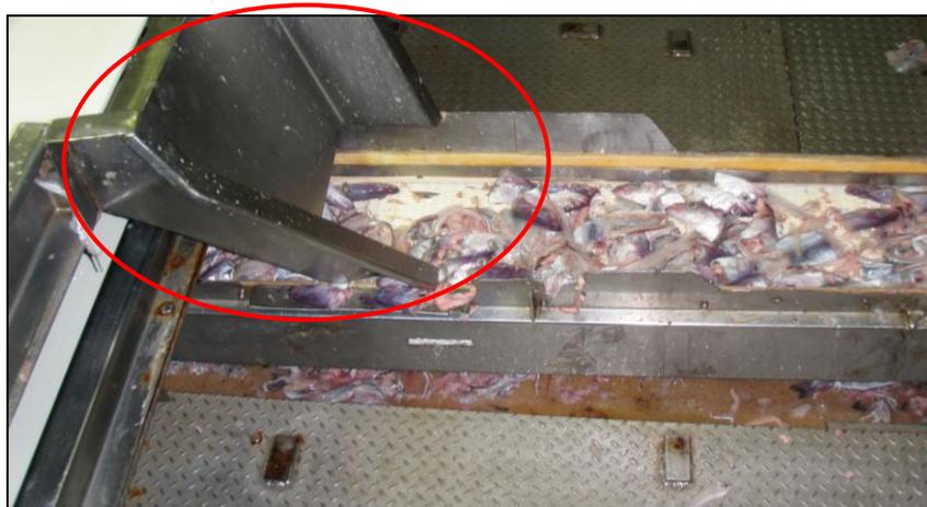
Figure 18 – Offal conveyor showing small chute from main conveyor
