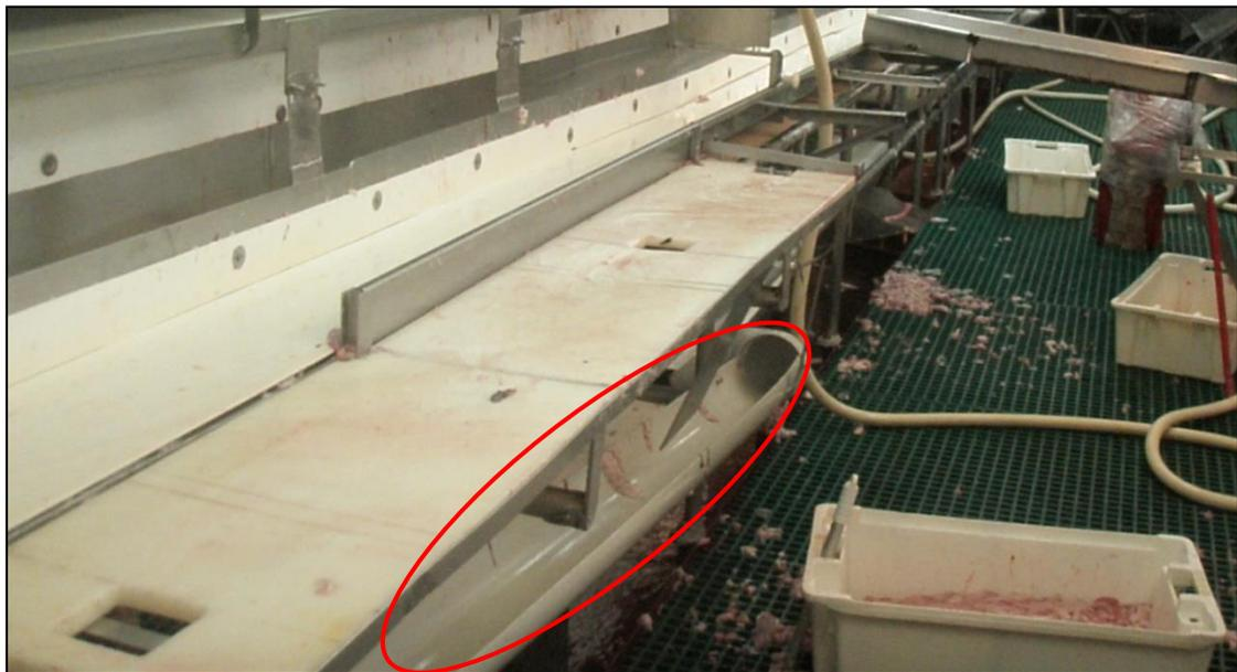
Figure 12 – chute from processing line to meal auger, enabling whole/processed fish to meal without quantification
