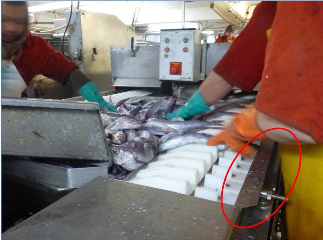
Figure 6 - Adjustable head rail on custom built machine
