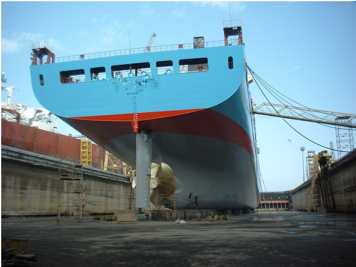
Figure 4: Example photograph showing propeller/ rudder size and configuration for a shipping container vessel of comparable size (292 m) and build to other vessels known to have traversed the location of the orca capture 10-50 hours prior to the capture event. (Note that this is not one of the actual vessels known to have traversed the area, because drydock photos of these particular vessels were not available.)
