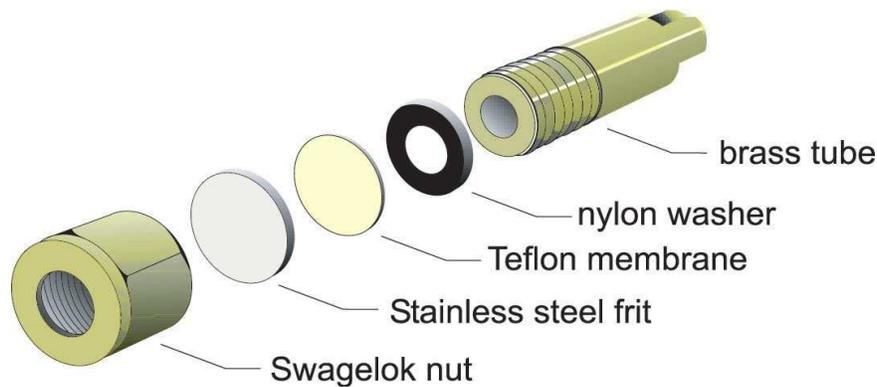
**Figure 3.** Exploded view of a permeation tube, taken from Lassey et al. (2001). The nylon washer was introduced into tubes filled from Dec 1998. Larger “cattle tubes” were first introduced in April 2000, prior to which two sheep tubes had been deployed in some experiments with cattle during 1999 and 2000.
