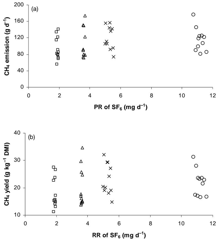
**Figure 10.** Estimated daily CH<sub>4</sub> emission (g d<sup>-1</sup>) (upper panel) and CH<sub>4</sub> yield (g kg(DMI)<sup>-1</sup>) (lower panel) as functions of SF<sub>6</sub> PR (mis-labelled RR in lower panel) (mg d<sup>-1</sup>) for individual animals for each PR treatment (low, □; medium, Δ; medium-high, ×; high, ○) in the “tailored experiment” of June 2005.
