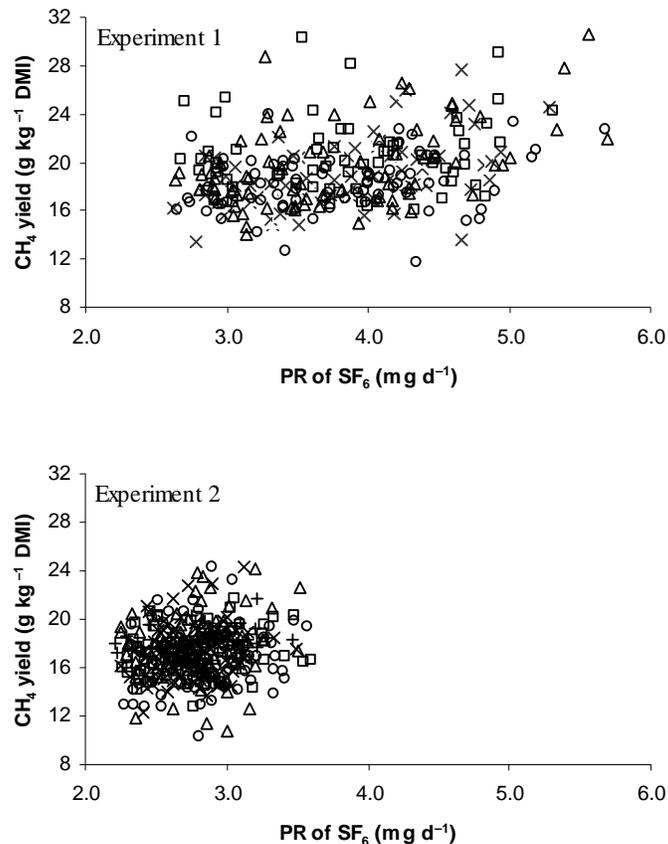
**Figure 9.** Relationships between estimated CH<sub>4</sub> yield (g(CH<sub>4</sub>) kg(DMI)<sup>-1</sup>) and SF<sub>6</sub> PR (mg(SF<sub>6</sub>) d<sup>-1</sup>) for each measurement group during grazing experiments 1 and 2. Labels x, □, △, ○, and + represent groups 1, 2, 3, 4 and 5, respectively.
