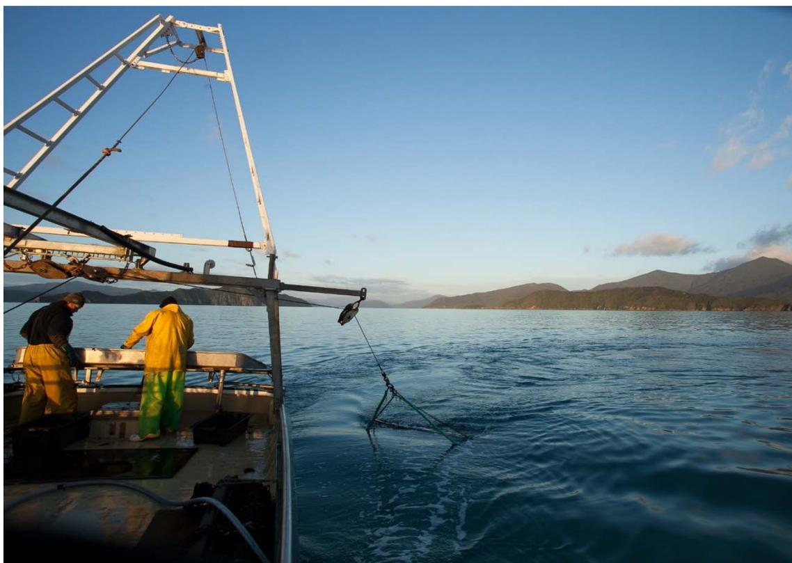
**Figure 4: Stern of FV *Okarito* showing deployment of ring-bag dredge in Marlborough Sounds. Photo credit: J. Williams.**
