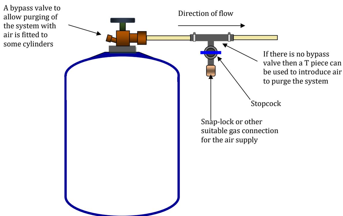
An alternative is to disconnect the supply pipe from the cylinder and force air down the pipe until all the methyl bromide has been forced into the enclosure.
