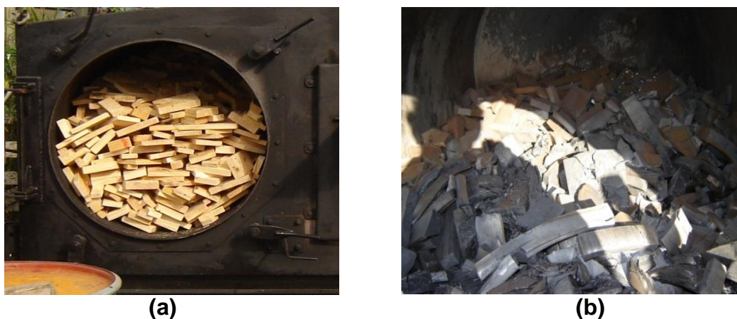
Figure 2.1 Kilnz Bio-energy retort filled with 180 kg of pine waste (a) and the charcoal after pyrolysis (b) prior to roller crushing.
