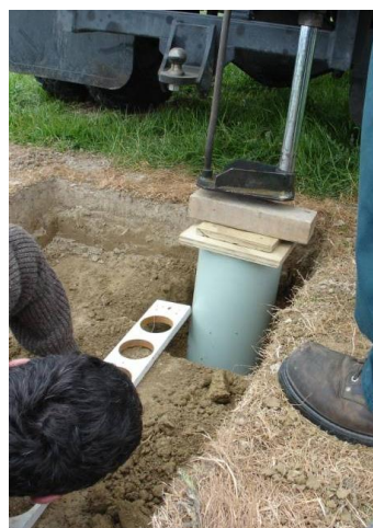
Photo 1.1 (Left) Details of how the intact soil cores (200–400 mm depth) were taken at the Tokomaru soil field site.
