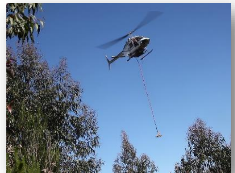
A helicopter delivers pesticide to one tree at a time
