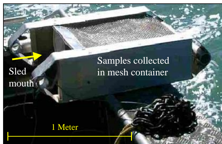
Figure 8: Ocklemann benthic sled for sampling epibenthos
