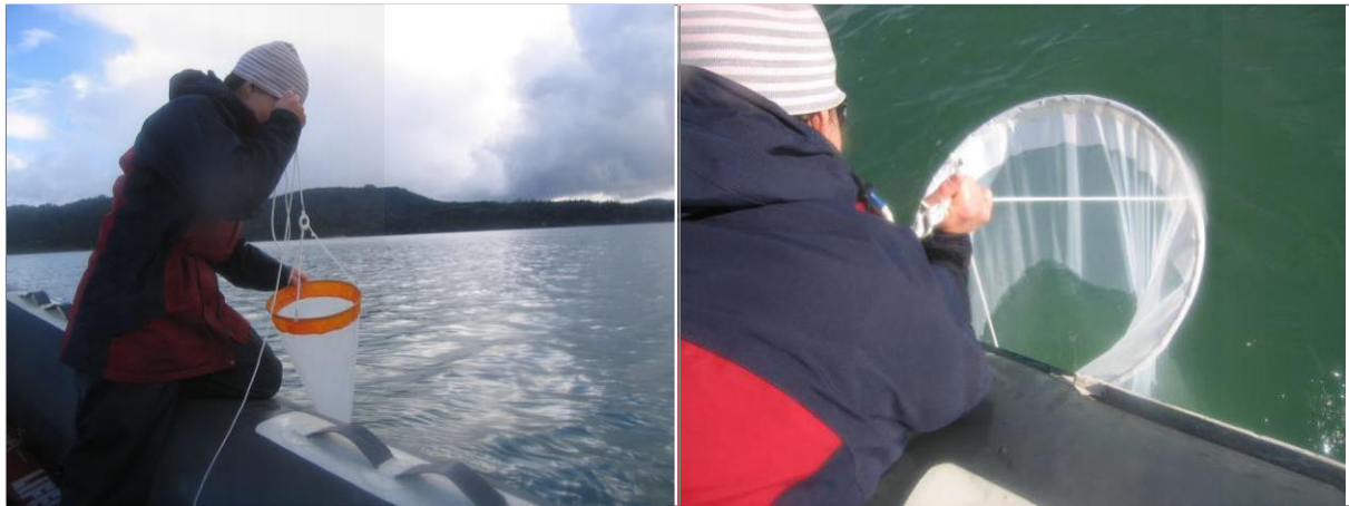
Figure 9: Field staff retrieving a plankton sample from a small net for phytoplankton (left) and a larger net for zooplankton (right).
