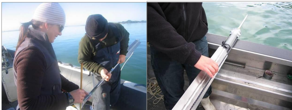
Figure 8: Field staff retrieving a sediment sample from the javelin core used for collection of dinoflagellate cyst samples during the Stewart Island survey, September 2006 (left). Additional weight was added for use in stronger currents (right).
