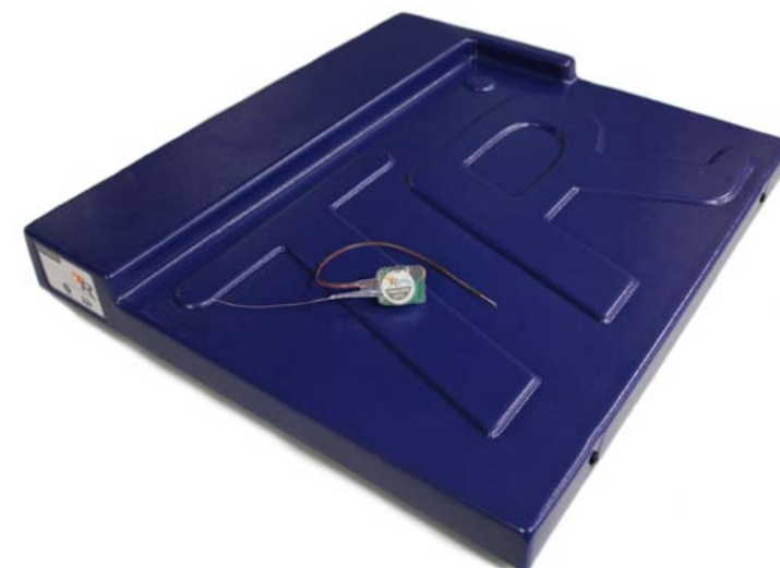
Telemeter for measuring blood pressure and ECG on the "SmartPad" that wirelessly receives the signals and recharges the battery
