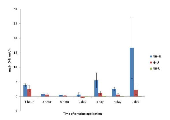
Figure 8: Nitrous oxide emissions after urine application. NH+U = urine added plots without herbage, H+U = urine added plots with herbage, NH-U = plots without herbage and without urine added. Error bars are standard error of mean (n=4).
