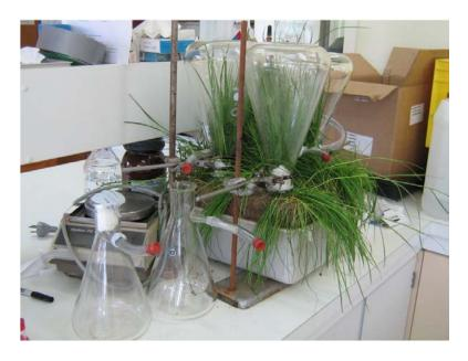
Figure 2: Laboratory set up to monitor  $N_2O$  emissions from intact leaves of pasture plants.
