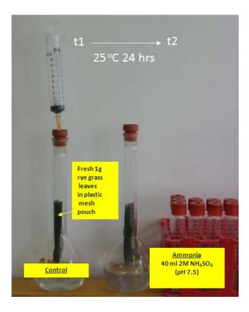
Figure 1: Experimental set up to detect  $N_2O$  emissions from detached leaves and detached leaves exposed to high ammonia ( $NH_3$ ) environments.
