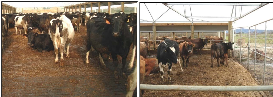
Figure 9: Left – cows in a Herd Home® in which the section of floor closest to the camera has been coated with a rubberised product; right – segregated calving pen in a Herd Home® shelter with extra space allowance and bedding (photos: Tom Pow, Herd Homes® Ltd)
