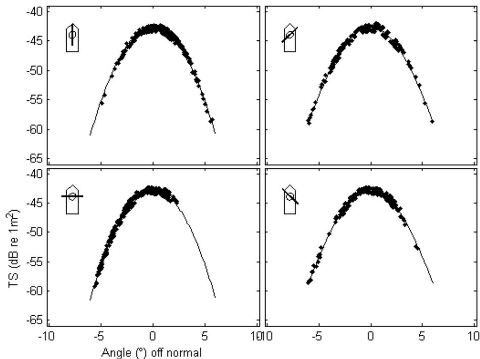
Figure A2.4. Beam pattern results from the calibration analysis for *Thomas Harrison* with 1.024 ms pulse length. The solid line is the theoretical beam pattern fit to the sphere echoes for four slices through the beam.
