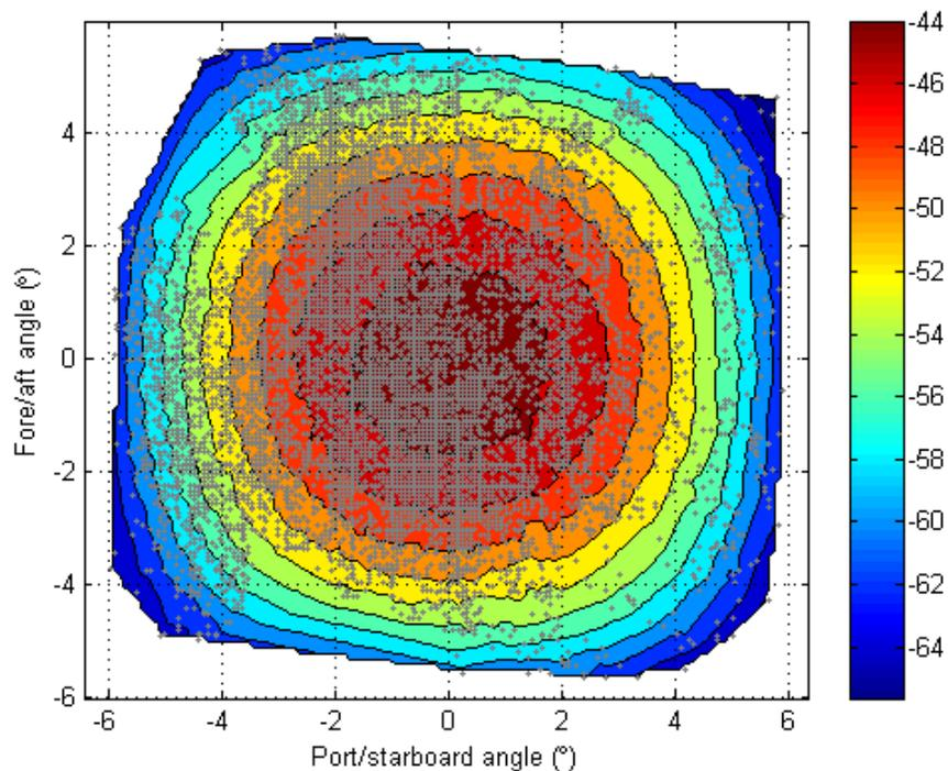
Figure A2.1. The estimated beam pattern from the sphere echo strength and position for the calibration of *Thomas Harrison* with 0.256 ms pulse length. The '+' symbols indicate where sphere echoes were received. The colours indicate the received sphere echo strength in dB re 1 m<sup>2</sup>.
