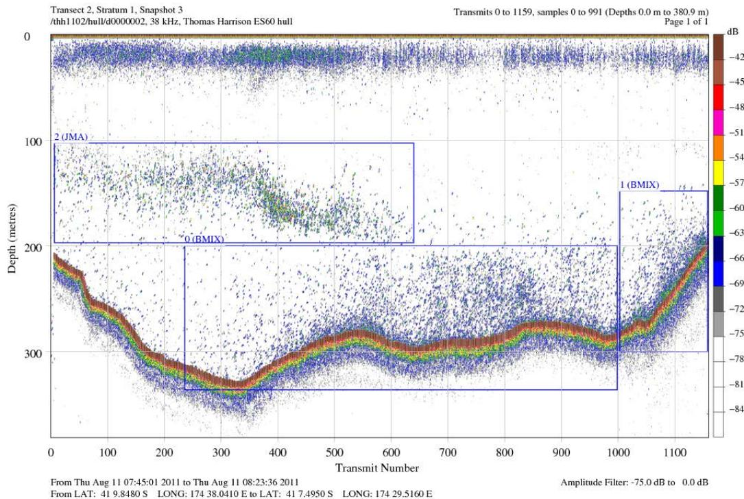
**Figure 8: Acoustic echogram from Narrows Basin (stratum 1) during snapshot 3 showing hoki bottom fuzz within 100 m of the bottom and jack mackerel above at 100–200 m. There is a pelagic layer within 50 m of the surface.**
