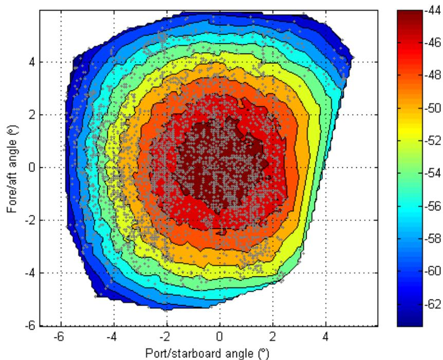
Figure A2.3. The estimated beam pattern from the sphere echo strength and position for the calibration of *Thomas Harrison* with 1.024 ms pulse length. The '+' symbols indicate where sphere echoes were received. The colours indicate the received sphere echo strength in dB re 1 m<sup>2</sup>.
