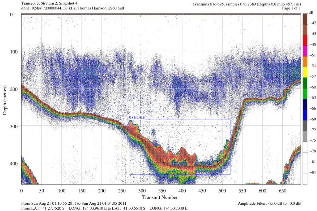
**Figure 5: Acoustic echogram from Cook Strait Canyon (stratum 2) during snapshot 4 showing a dense hoki school close to the bottom at night. The dispersed layer from 130 to 250 m is probably mesopelagic fish.**
