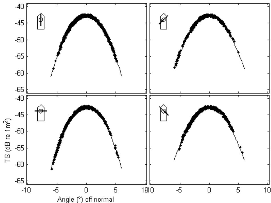
Figure A2.2. Beam pattern results from the calibration analysis for *Thomas Harrison* with 0.256 ms pulse length. The solid line is the theoretical beam pattern fit to the sphere echoes for four slices through the beam.
