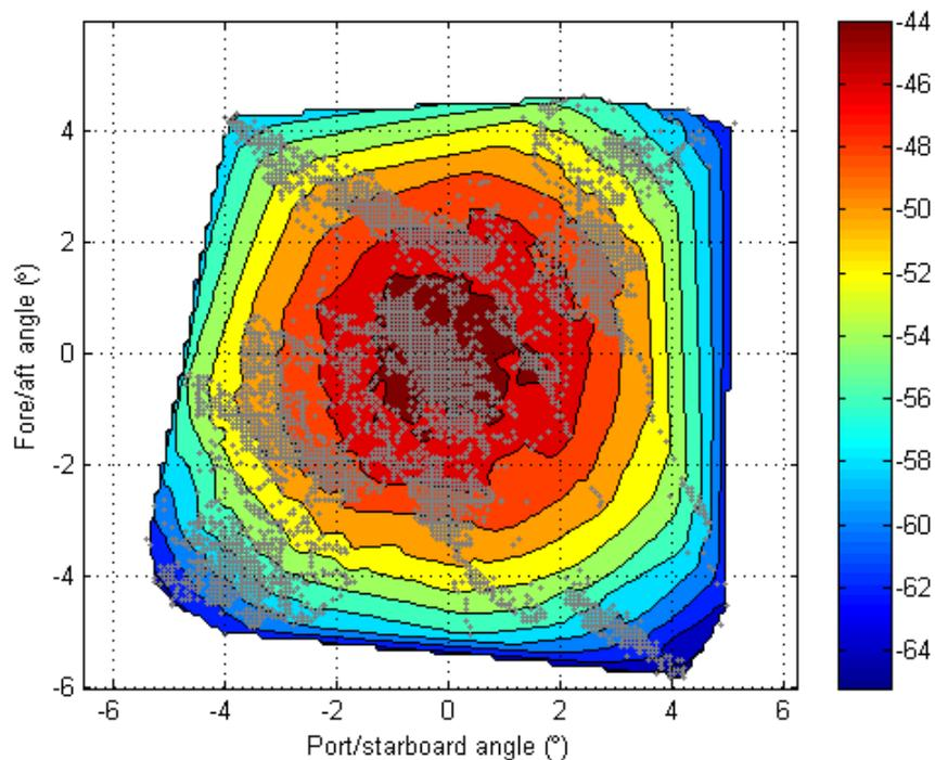
Figure A1.1. The estimated beam pattern from the sphere echo strength and position for the calibration of *Independent 1*. The '+' symbols indicate where sphere echoes were received. The colours indicate the received sphere echo strength in dB re 1 m<sup>2</sup>.
