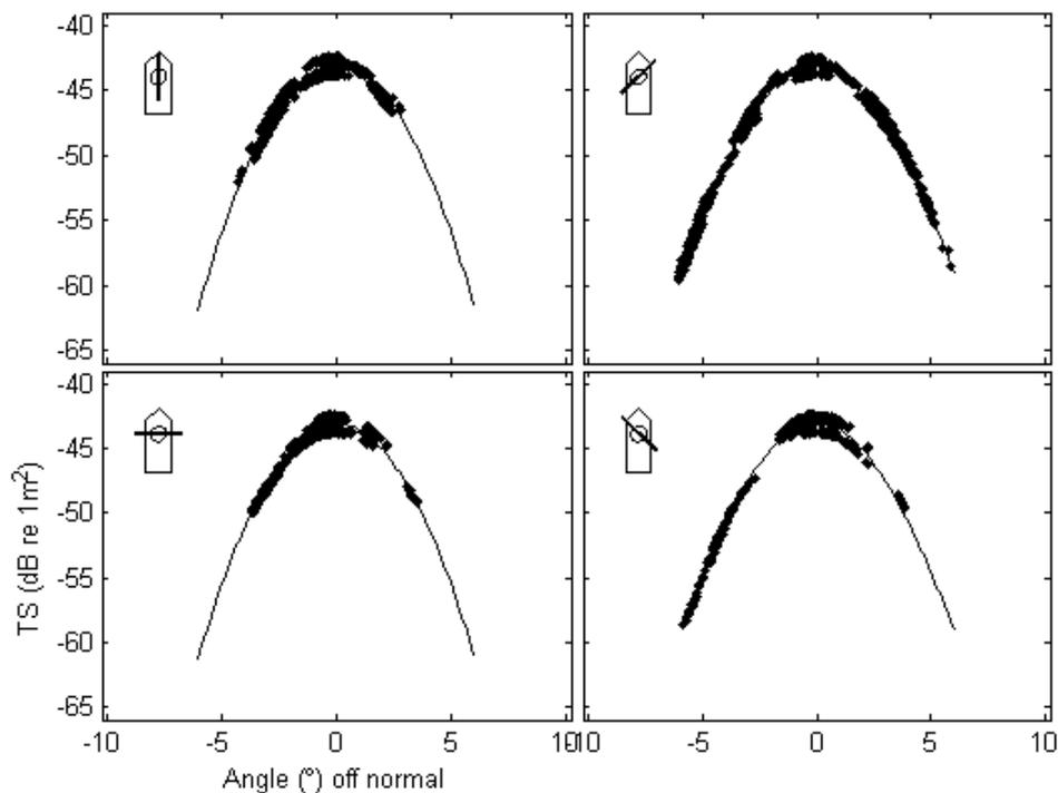
Figure A1.2. Beam pattern results from the calibration analysis for *Independent 1*. The solid line is the theoretical beam pattern fit to the sphere echoes for four slices through the beam.
