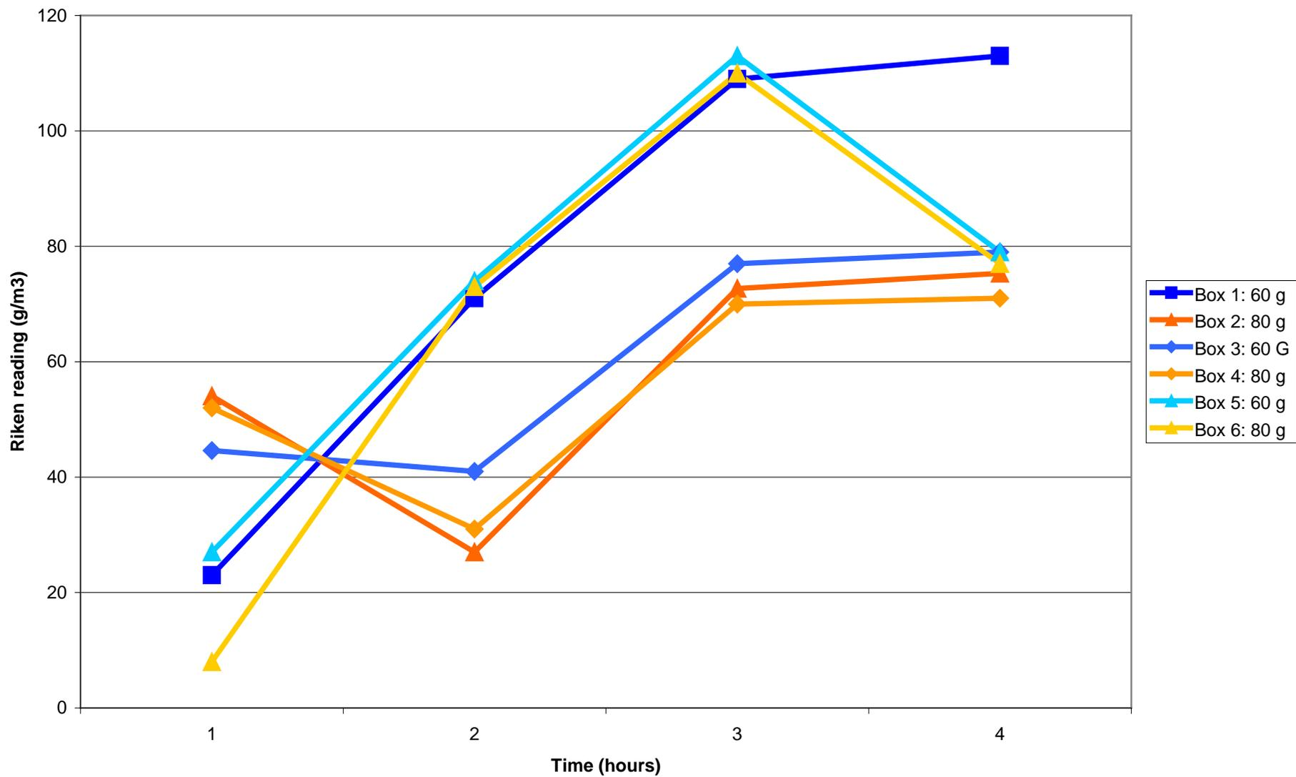
**Figure 8: Comparison of fumigant levels between test RFRs for first four hours following fumigation.**
