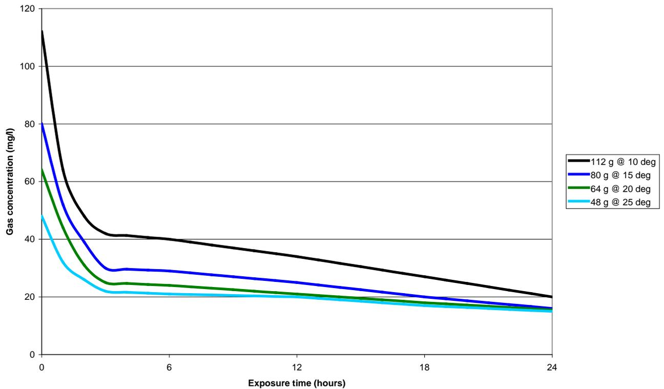
**Figure 9: Theoretical progressive gas concentrations with 50% loading on container (based on Kawakami 2007).**
