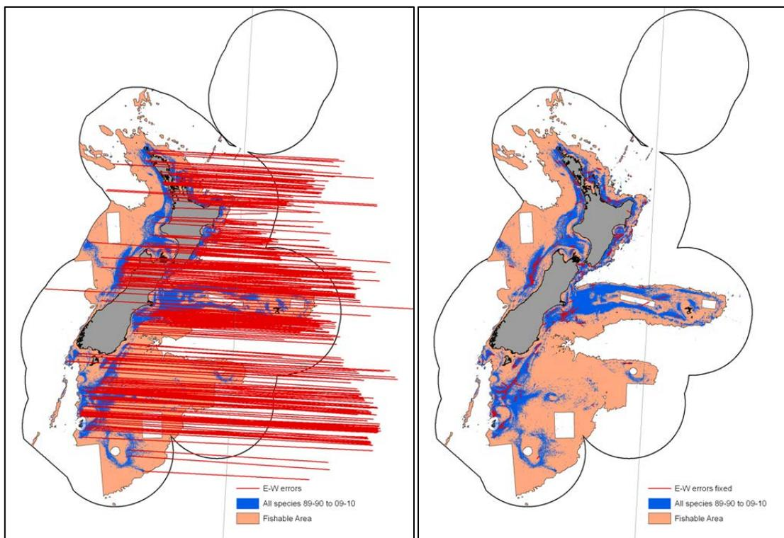
**Figure 4: Maps displaying the 419 tows (red lines) corrected for an east-west longitude error. Before correction (left) and after correction (right). The majority of the corrected tows lie inside the estimated swept area, and all lie inside the Fishable Area.**
