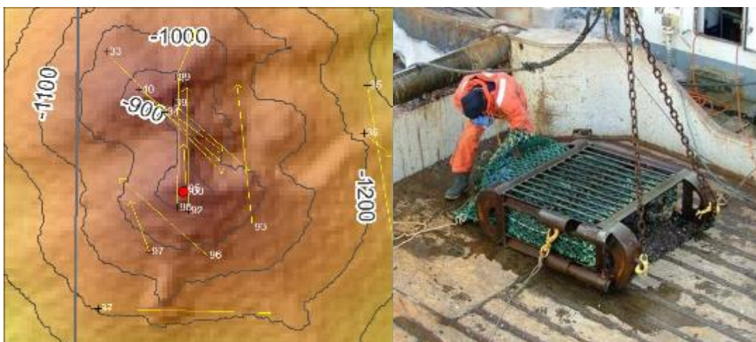
Figure 7.3a (left image): DTIS Transect lines and benthic sled tow lines (in yellow) on Clark Seamount, southern end of Kermadec Arc. Red dot marks the position of the CTD, adjacent to station 95 where live corals were sampled. Figure 7.3b (right image): Benthic sled invertebrate sampling tool. Both images taken during voyage, TAN1205 (Images Malcolm Clark (NIWA)).
