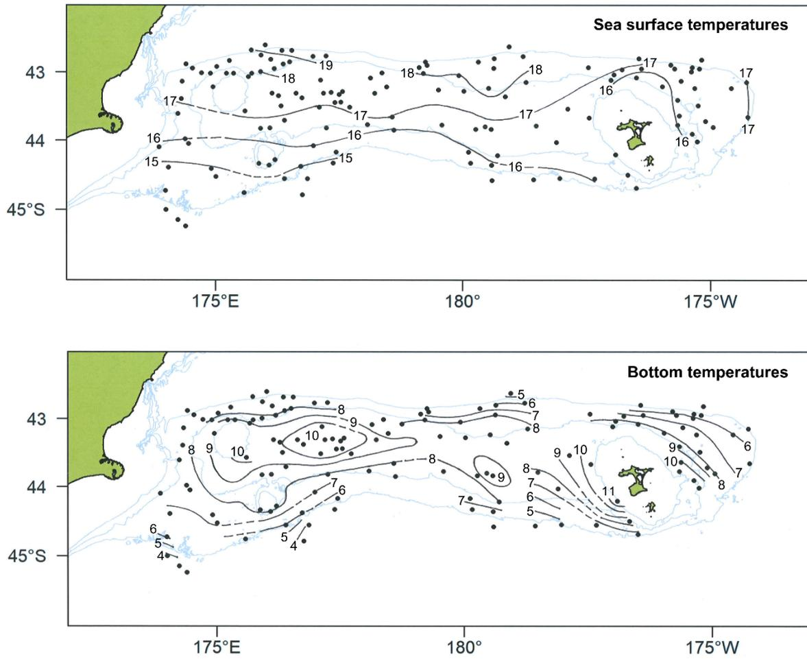
**Figure 3: Positions of sea surface and bottom temperature recordings and approximate location of isotherms (°C), interpolated by eye, for TAN2201. The temperatures shown are from the calibrated Seabird CTD recordings made during each tow.**
