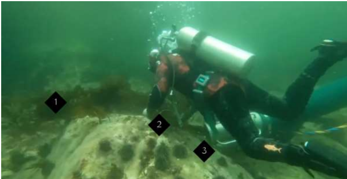
Figure 4: Underwater operation of the suction dredge: 1) U. pinnatifida plants (still attached); 2) Diver removing U. pinnatifida from the reef; 3) Suction dredge nozzle where plants are fed for transport to the surface.
