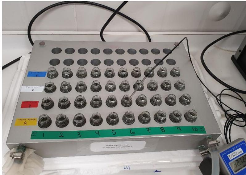
Figure 7. Aluminium block used to assess the sensitivity of embryos to a range of temperatures. Photo credit: Cawthron Institute.
