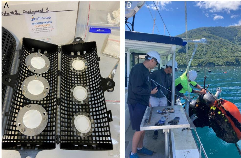
Figure 4. (A) Berley cage used to deploy passive samplers (B) out on the mussel longlines. Photo credits: Julien Vignier, Cawthron Institute.
