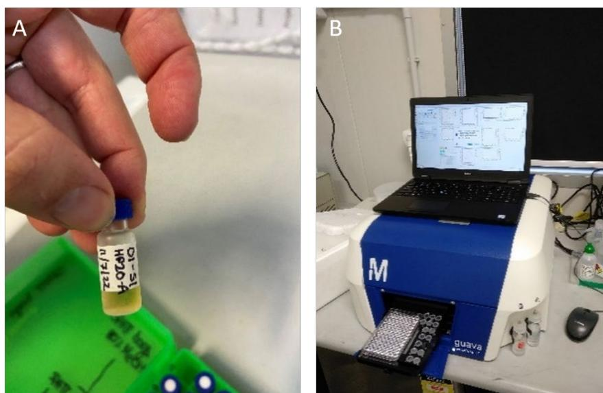
Figure 10. (A) Field-collected extract consisting of a cocktail of organic contaminants to be tested on Greenshell™ mussel sperm. (B) Guava® flow cytometer used for high-throughput cellular assessments of exposed sperm. Photo credits: Julien Vignier, Cawthron Institute.
