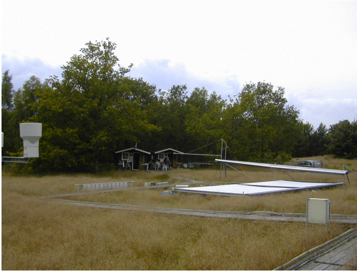
Plate 2 Passive warming screen extended above heathland in the CLIMAITE experiment, Denmark (Mikkelesen et al 2008).
