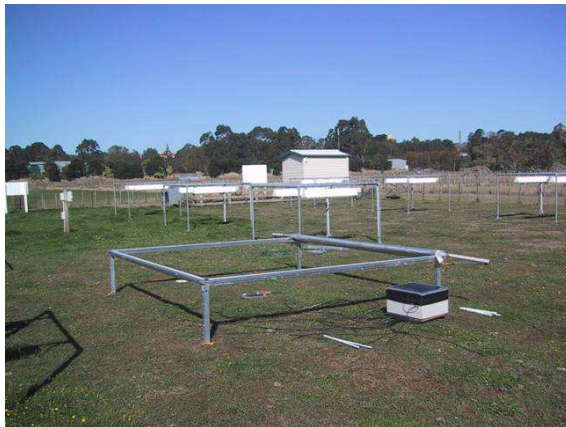
Plate 3 Prototype passive warming screen open (left) and closed (right). Solar powered data logger and sensor cables also visible. Test location: Agresearch Grasslands, Palmerston North.
