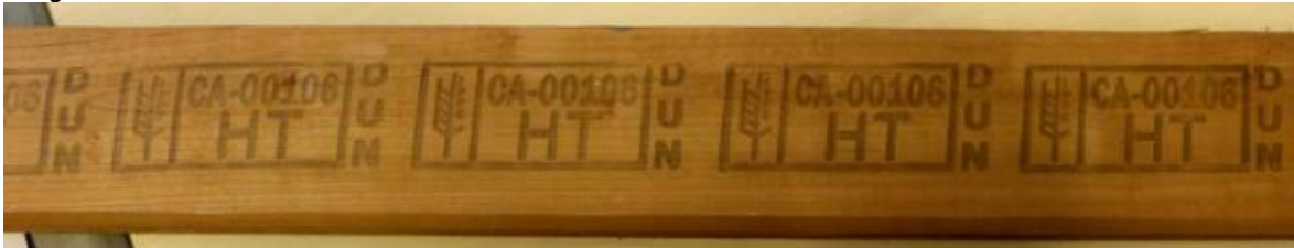
Image 4. Roll mark with additional information included outside the borders of the mark.
