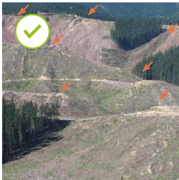
Planning for centralised and two-stage processing almost eliminated landing slash, significantly reduced landing size (orange arrows), and removed a potential fire risk in this highly erosion-prone and summer-dry hill country.
