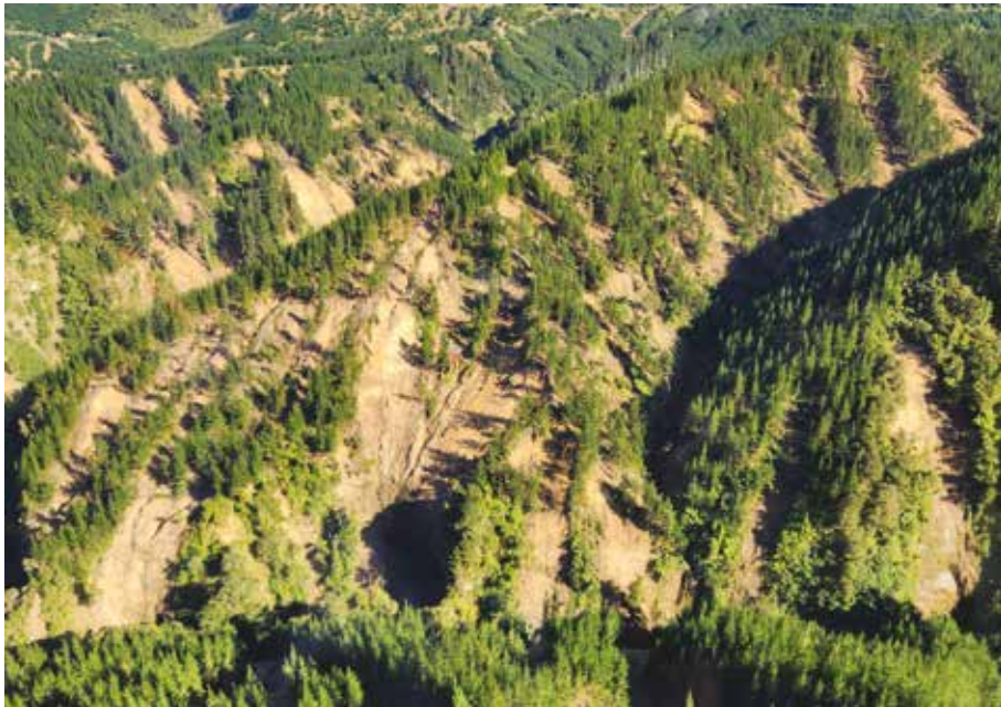
Bedrock failure in mid-rotation forest created a debris avalanche in Hawke's Bay. Both images are post-Cyclone Gabrielle 2023.
