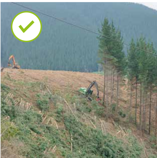
Left: An advantage of mechanised harvesting over manual harvesting is reduced breakage. A winch-assisted felling machine directionally falls trees and bunches them aligned in the direction they will be hauled to a landing.
