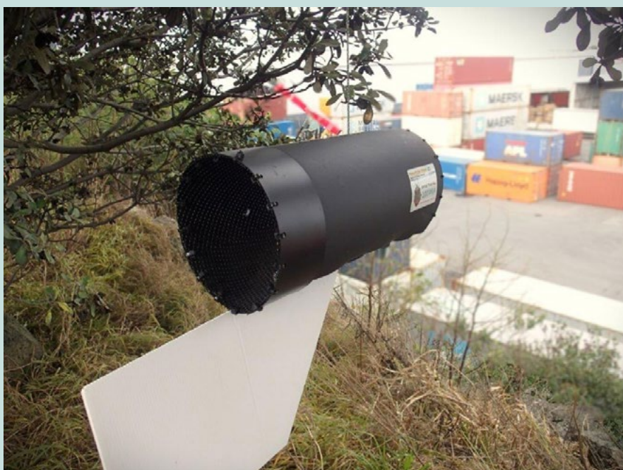
Figure 5: Aerodynamic BMSB trap
