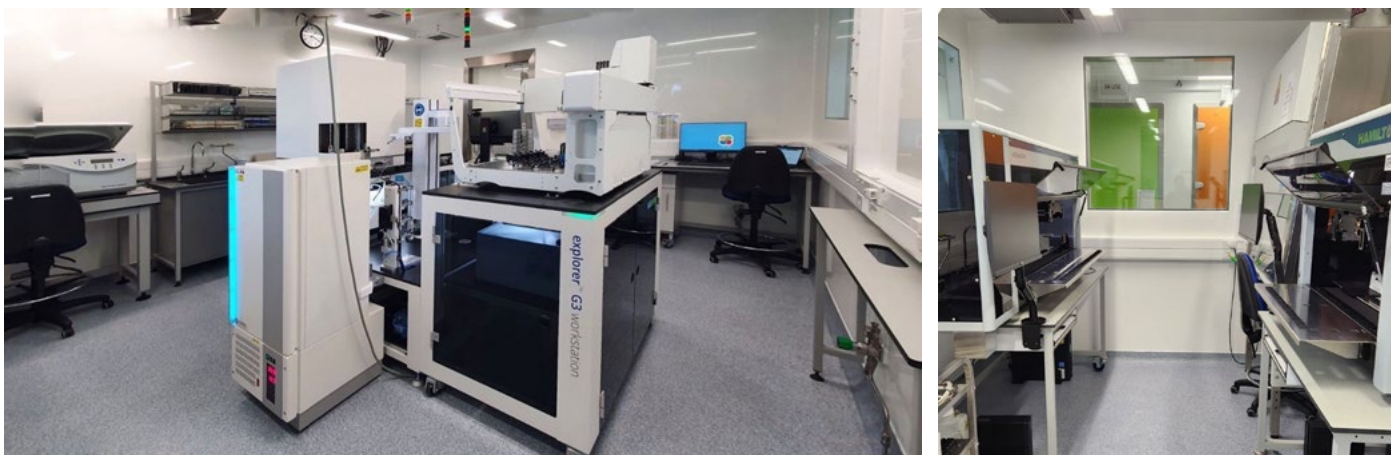
Figure 4: (A) ELISA Robot – The Explorer G3 Workstation; (B) PCR Robots – Hamilton Star and Starlet
