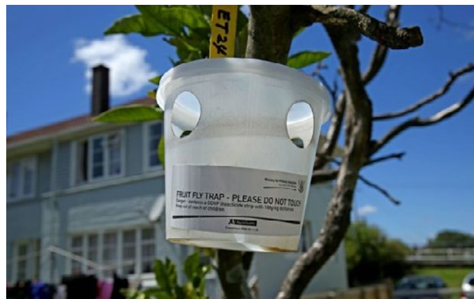
Figure 3: A Lynfield trap used to catch male fruit flies. Photo: ASUREQuality
