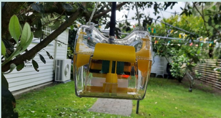
Figure 5: A RapidAIM© automated fruit fly trap unit
