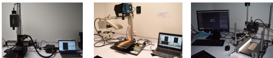
Figure 2 – Three hyperspectral systems most used in the study, from left to right: Resonon, Headwall and Snapscan.
