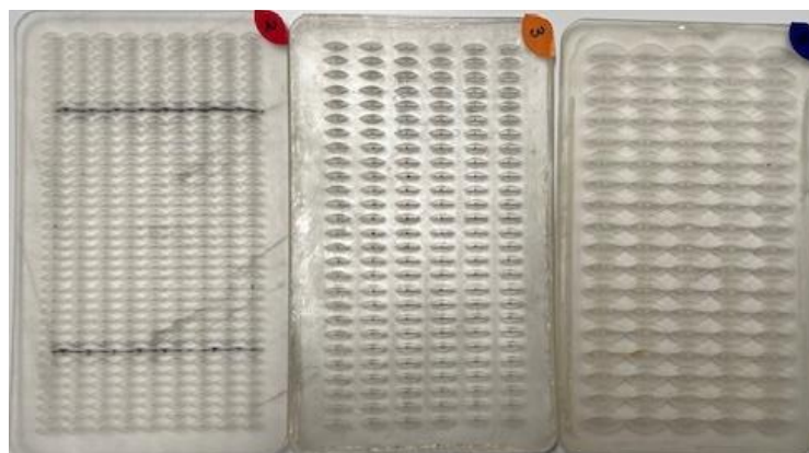
Figure 4 - Seed tray on vacuum frame. A vacuum pump applies negative pressure resulting in seeds being sucked into the wells. If seeds are too small and fall through the wells, they are captured in the box by filter paper on the outlet and identified by seed technicians. This separates seeds mostly into individual wells. The seed trays are software generated for any seed dimensions and shapes.
