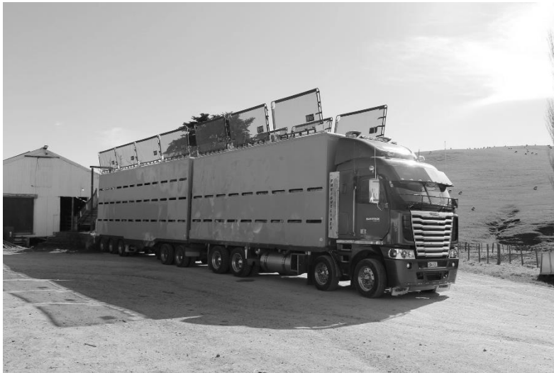
Figure 23. Livestock crate fitted with the CrateSafe™ covers. Photo provided by Landquip, NZ.
