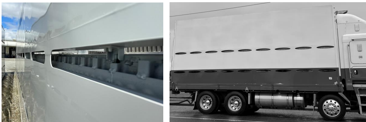
Figure 6. Oval ventilation holes running along the side of a newly built livestock crate (left). Note that the floor folded against the wall is blocking the ventilation gap in both photos.
