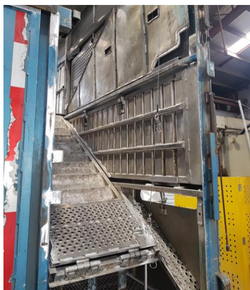
Figure 33. Winch operated ramp to mechanically lift/move the internal ramp and reduce the risk of injuries.
