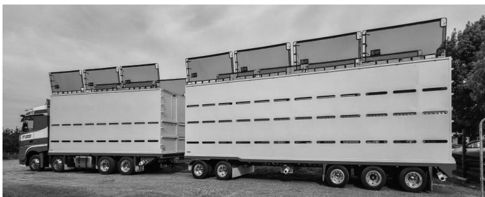
Figure 31. A CrateSafe™ system installed on the top of NZ crate for driver safety when working on top of the crates, also ensuring that covers are utilised as required. Photos provided by Landquip, NZ.
