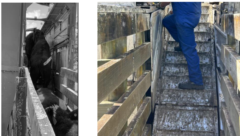
Figure 27. Driver setting up the internal ramp for loading and beef cattle being loaded onto the top deck.
