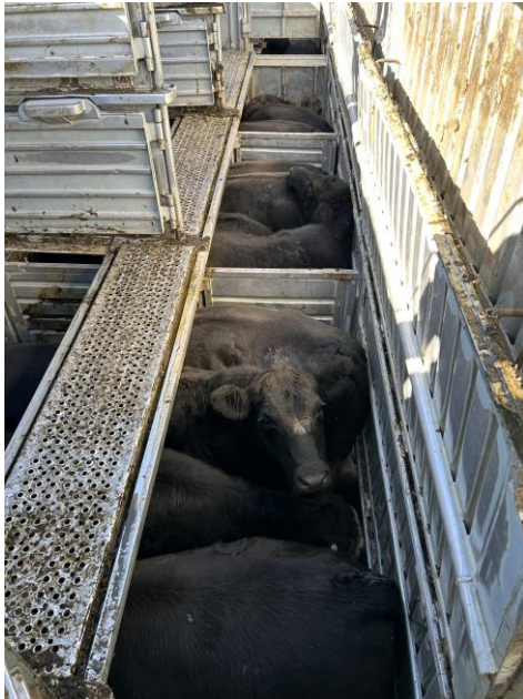
Figure 20. Steers (approximately 600kgs) loaded (4/pen) into the lower deck of a two-deck crate configuration before and after the floors were closed down.
