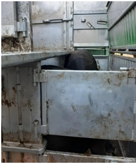
Figure 14. The back of a cattle beast touching the ceiling before the floors were folded down in a NZ livestock crate.
