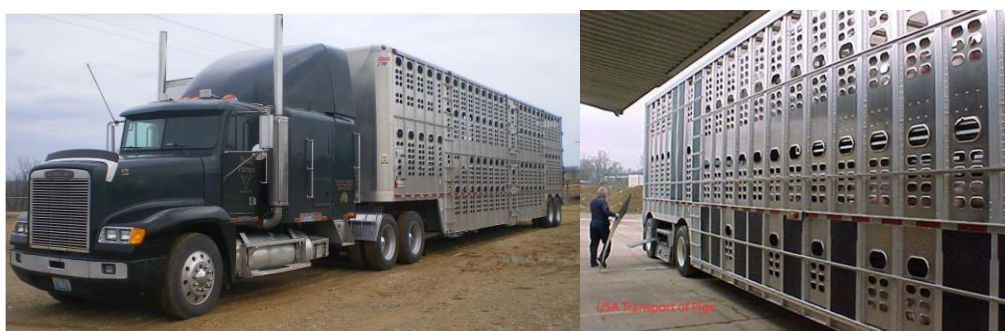
Figure 11. Pot-bellied vehicles, typically used for pig transport in USA, showing the greater amount of ventilation compared to NZ livestock crates.
