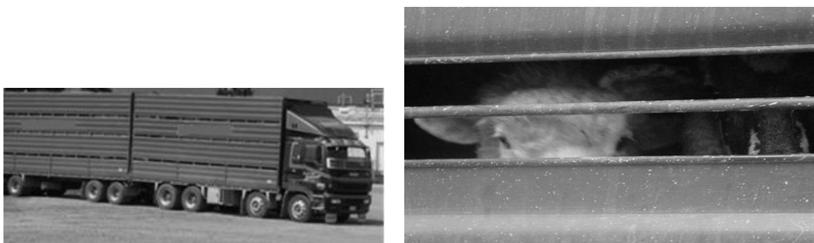
Figure 7. Ventilation gaps in older NZ livestock crates with continuous openings along the sides of the crate.
