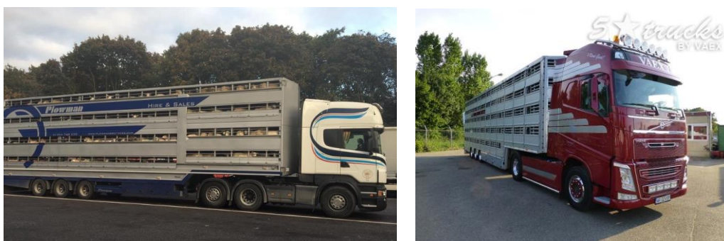
Figure 8. Example of livestock crates in UK showing a greater amount of ventilation compared to NZ livestock crates.
