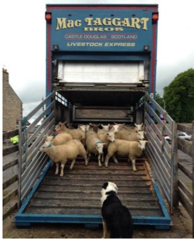
Figure 25. An example of a UK crate design with a wide ramp and entry for loading and unloading.
