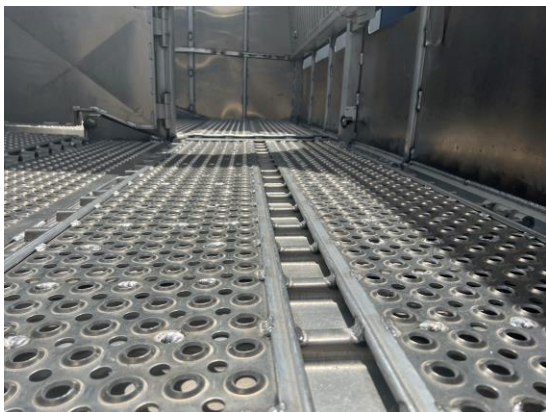
Figure 29. Perforated aluminium floor on the second deck of a new NZ livestock crate.
