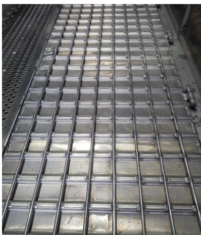
Figure 30. Grip bars (115mm gap) incorporated into the top deck of a new two-deck cattle livestock crate in NZ.
