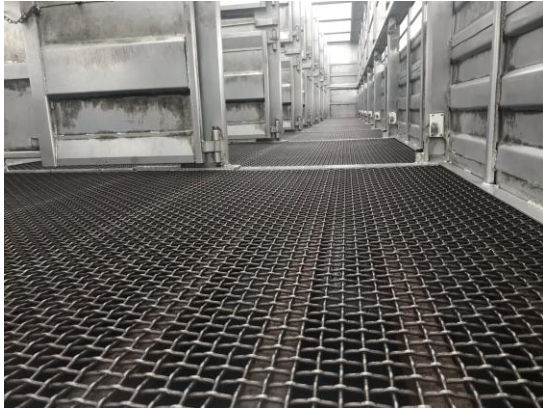
Figure 28. Steel mesh floor on the bottom deck of a new NZ livestock crate.
