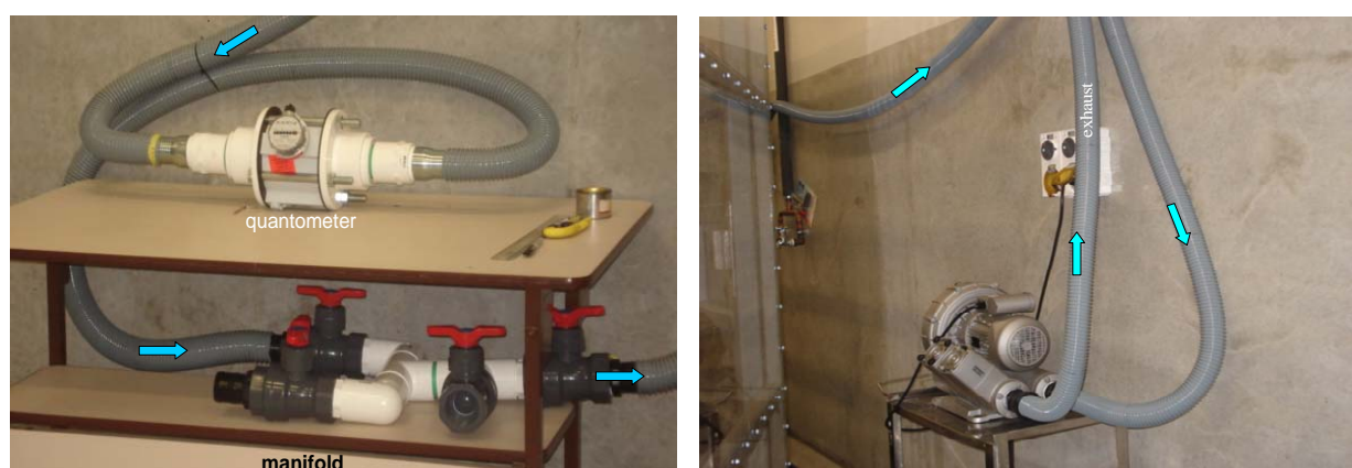
Fig 12. Cattle calorimetry system: gas quantometer and manifold, and the side-channel vacuum pump. Arrows indicate direction of gas flow.
