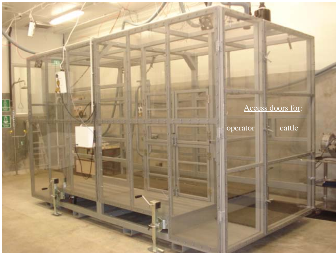
Fig. 10. Cattle calorimetry chamber showing its structural metal frame and clear walls and roof
