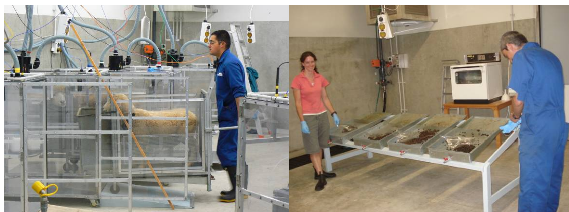
Fig.2. Sheep are housed in modified metabolic crates with faecal and urine collection trays. The transparent walls of chambers enable the sheep to acclimatise to the system almost immediately, as shown by their eating, ruminating and lying behaviour.
