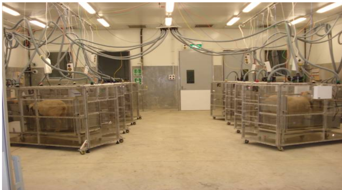
Fig 1. The sheep calorimetry facility at AgResearch Grasslands. The newly built 4 chambers (to the right) and the previously existing 4-chamber facility (to the left) are managed as sub-units (for purposes of air circulation only), and integrated into an 8-chamber facility. Fresh air is sourced from a common vent in the building ceiling.
