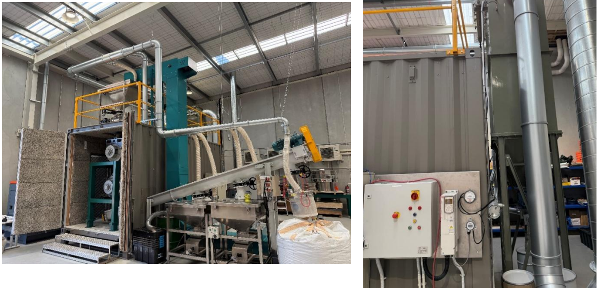
Figure 6. Pilot scale dust suppression system evaluated in this programme.
