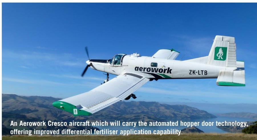
An Aerowork Cresco aircraft which will carry the automated hopper door technology, offering improved differential fertiliser application capability
