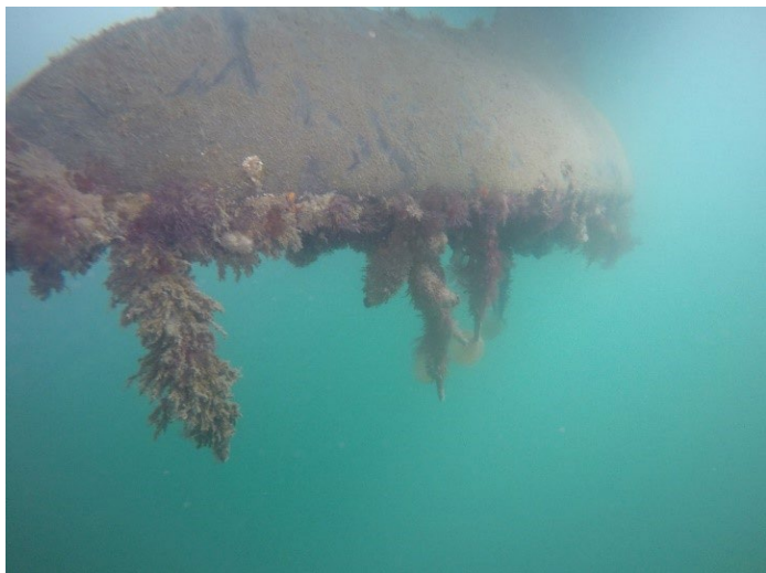
The bottom of the keel bulb of this yacht wasn't cleaned properly before departing from Auckland. Several fan worms and other marine pests were allowed to grow as a consequence. (Photo: NZ Diving and Salvage)
